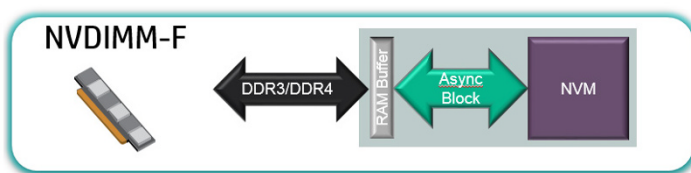
Figure 2-2: The NVDIMM-F module.
