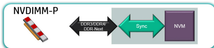
Figure 2-3: A NVDIMM-P module.
