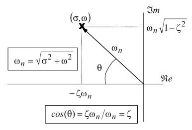
o The damping ratio is calculated as  $\zeta = cos(\theta)$ . For example, poles that lie below the  $\theta = 45^{\circ}$  line have damping ratios  $\zeta > 0.7$ . See the diagram below.
