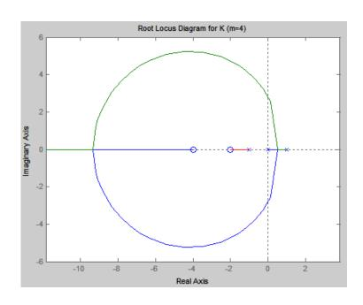
Note that MATLAB does not show the direction of the movement of the poles. It is understood that the movement is from the *poles to the zeros of* P(s). The "axis" command ensures that the diagram is shown in its *true shape*.
