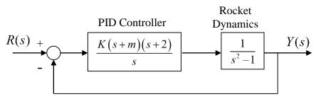
The characteristic equation of the closed-loop system is 1+GH(s)=0 or 1+KP(s)=0. Substituting the transfer functions from the block diagram gives
