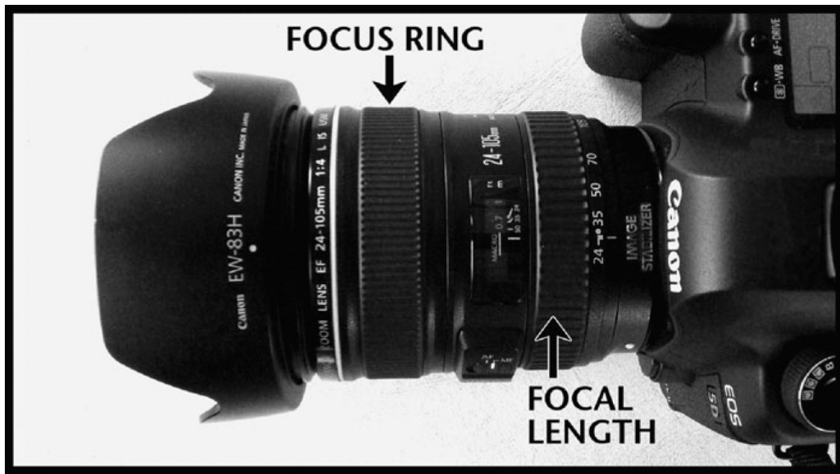
FIGURE 2.13 A camera lens with zoom or varifocal capabilities.
