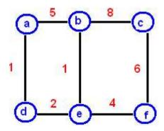
One cycle is a b c f e d a that has a total weight 26. Is there a shorter cycle?
