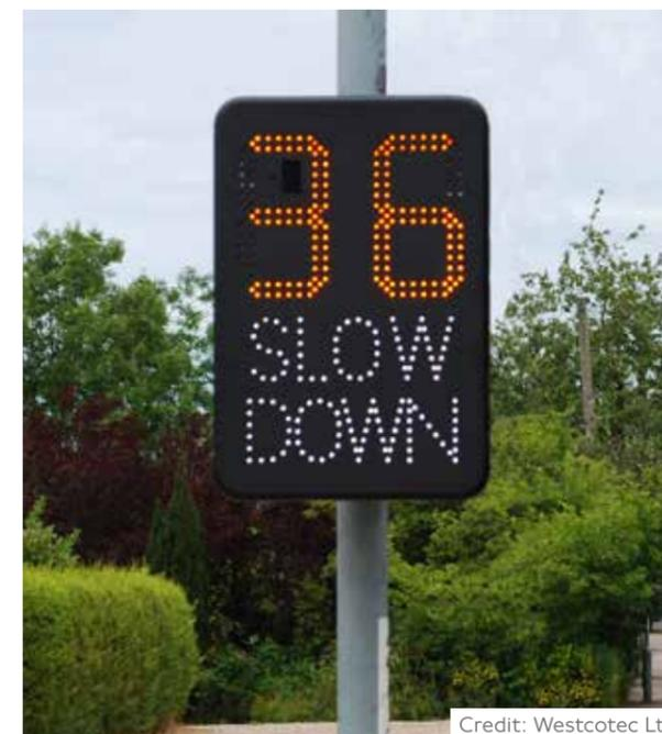
Speed indicator device showing speed and warning message
