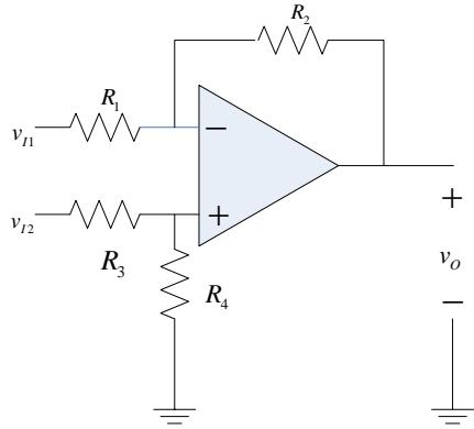
Q1.(D2.16) Find values for resistance in above circuit, so that the circuit behaves as a difference amplifier with an input resistance of  $20\text{ k}\Omega$  and a gain of 10.
