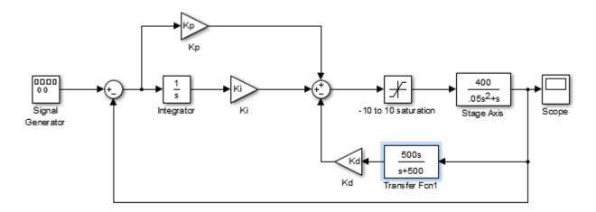
The  $\frac{500s}{s+500}$  transfer function is estimating the derivative. (The true derivative "s" is impossible to implement.) The 500 is a tunable gain causing the derivative approximation to perform differently. You should not have to change this 500 value because it has already been tested to work well with the XY stage sampling the feedback every 1 millisecond. You will however want to tune the Kd gain.
