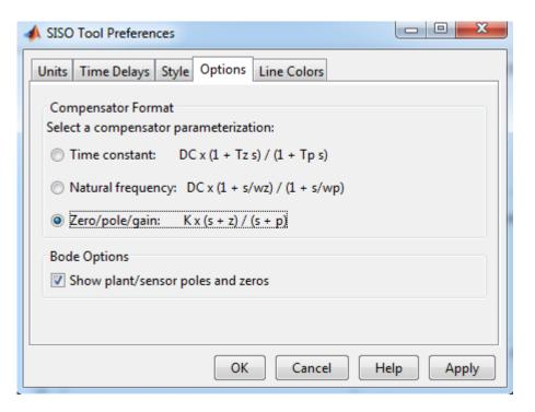
C2 is straight forward to setup by assigning it a real pole at -500 and real zero at zero. Then the gain of C2 is Kd\*500. Start the Kd gain at 0.006 for your first iteration.
