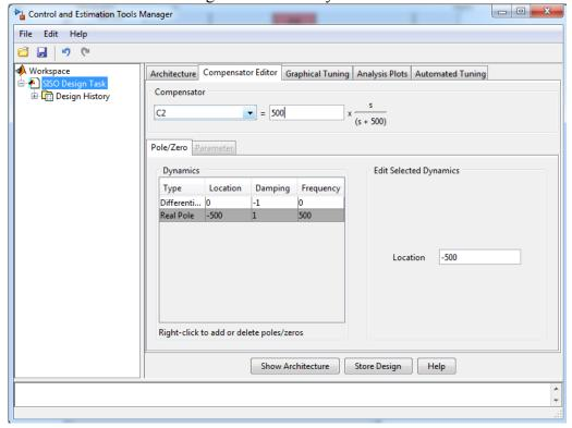
For the error path what are the poles and zeros of C1 that has the transfer function  $Kp + \frac{Ki}{s}$ . Show that this transfer function can be rewritten as  $Kp * \frac{s + \frac{Ki}{Kp}}{s}$ . So in C1 add a real pole at zero and a real zero.
