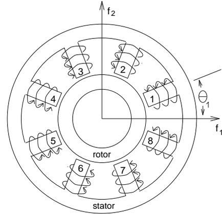
Figure 1: 8-pole heteropolar radial magnetic bearing
