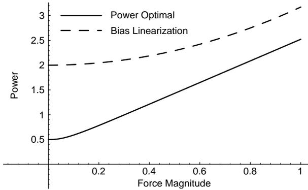
Figure 5: Power optimal and bias linearization power consumption.
