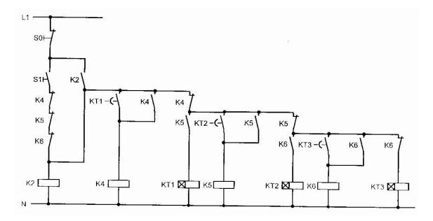
Complete the function diagram and draw up an assignment list for using the PLC as a control unit.
