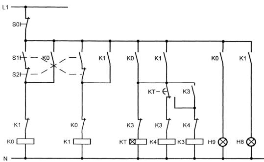
The mains contactor K0 is activated for clockwise rotation of the motor by actuating pushbutton S1. K0 is self-holding. For counterclockwise rotation the mains contactor K1 is activated by pressing pushbutton S2. K1 is self-holding. Both contactors are interlocked, i.e. pushbutton and contactor are latched.
