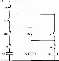
All of the controls for star-delta circuits must fundamentally be designed so that during switchover from star to delta, the star contactor must deactivate first, before the delta contactor may be activated. Otherwise switching overlaps cause short-circuits in the main circuit.
