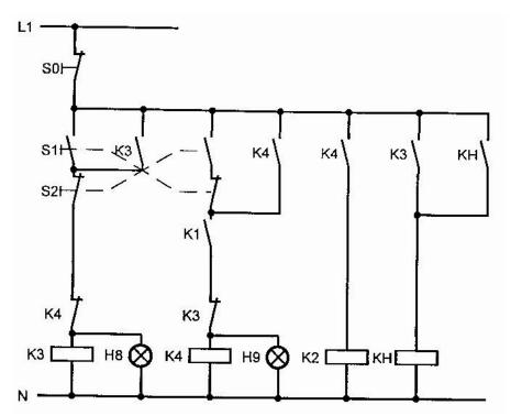
Complete the following function diagram and make an assignment list for your PLC. The indicator lamps H8 and H9 should be triggered parallel to contactors K3 and K4. The auxiliary contactor KH is realized within the PLC control program using a marker.
