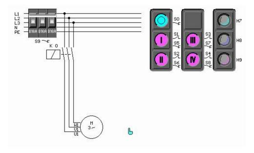
The circuit with a storage function in a contactor control operation is called the self-holding circuit. An NO contact of the contactor is connected parallel to the onbutton as a self-holding contact. An NC contact is used as the off-button, which interrupts the holding current circuit when activated and thus cancels the self-holding action.
