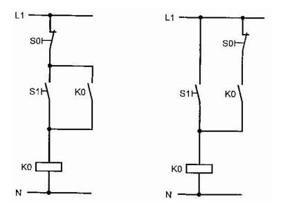
The two circuit diagrams should not be converted into function diagrams. Since the S0 is designed as an NC contact, it must be polled for 1-signals. Correctly complete the function diagram on the right.
