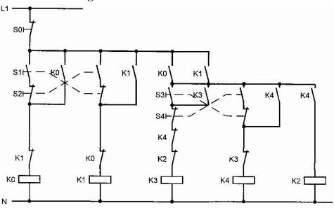
After determining the rotation direction, the low or the high speed is switched on each time from 0. Switchover from a low initial speed setting to the high speed should be possible, but switching the setting back from the high to the low speed should not. Reversal of rotation direction and switch back to low speed are only possible if the motor has been switched off first.
