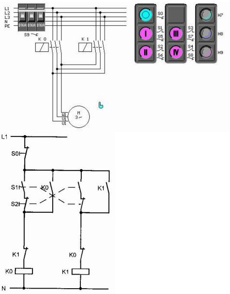
The pushbuttons and the contactors are interlocked (latching). For pushbutton latching there are two different possibilities:
