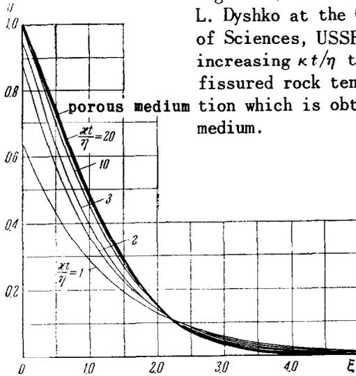
as a function of the self-similar variable  $\xi$  in Fig. 2. (The calculations were carried out by A. L. Dyshko at the Computing Center of the Academy of Sciences, USSR). It can be seen that with increasing  $\kappa t/\eta$  the pressure distribution in a fissured rock tends to the self-similar distribution which is obtained in an ordinary porous medium.
