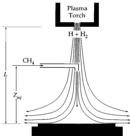
FIG. 1. Schematic diagram of the plasma torch/substrate configuration. Methane is injected into a mixture of H and H<sub>2</sub>, which exit the torch at 2500 K and a velocity of  $2 \times 10^5$  cm/s.
