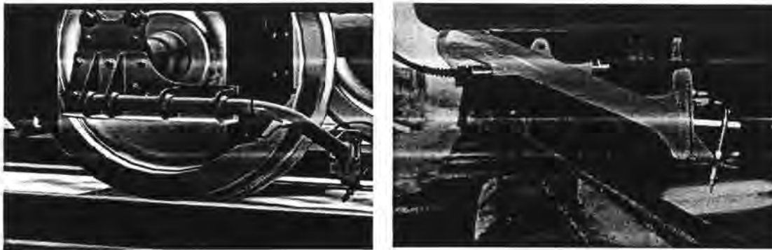
Figure 5 - LUL designed spray mounting bracket - CAD representation (left) and actual installation (right)
