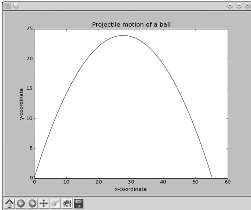
Figure 2-14: The trajectory of a ball when thrown with a velocity of 25 m/s at an angle of 60 degrees
