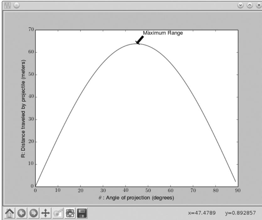
Figure 7-4: The range of a projectile thrown with an initial velocity of 25 m/s with varying angles of projection
