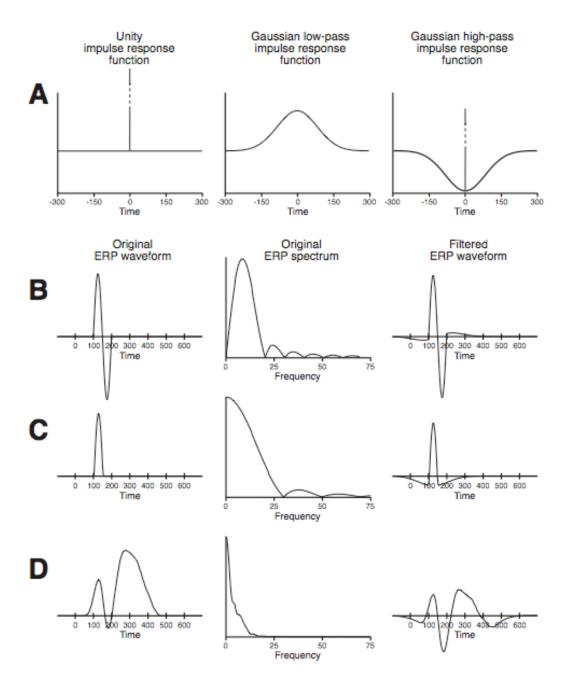
Figure 5.10. Construction and application of a gaussian high-pass filter. (A) A unity impulse response function multiplied by a gaussian low-pass impulse response function yields a gaussian high-pass impulse response function. (B), (C), and (D) show the application of this filter to three different ERP waveforms.
