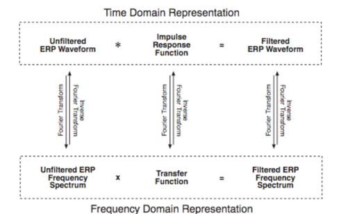
Figure 5.6. Relationship between filtering in the time and frequency domains, showing: (1) that each term in the time domain can be converted to a corresponding term in the frequency domain by means of the fourier transform; and (2) that convolution (represented by the \* operator) in the time domain is equivalent to multiplication (represented by the X operator) in the frequency domain.
