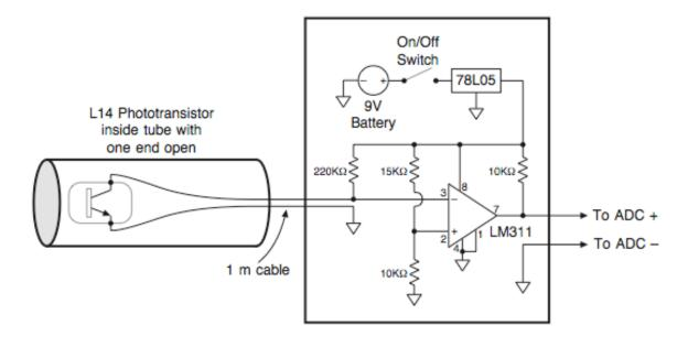
Figure 8.2. A circuit that can be used to measure the light emitted by a small region of a video display. The output can be connected directly to the analog-to-digital converter of your EEG digitization system (assuming that the voltage range is correct). Thanks to Lloyd Frei for designing this circuit.
