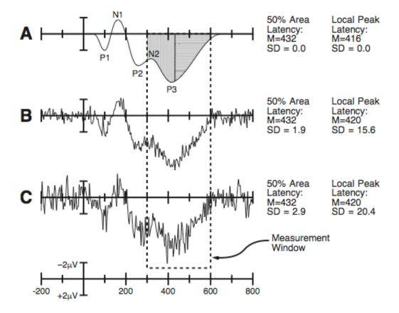
Figure 6.3. Application of 50% area latency and local peak latency measures to a noise-free ERP waveform (A), an ERP waveform with a moderate amount of noise (B), and an ERP waveform with significant noise (C). In each case, measurements were obtained from 100 waveforms, and the mean (M) and standard deviation (SD) across these 100 measures are shown. Negative is plotted upwards.
