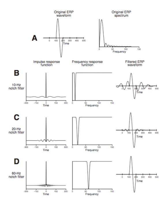
Figure 5.8. Examples of temporal distortions produced by notch filters. The original artificial ERP waveform (one cycle of a 10 Hz sine wave) and its fourier transform are shown in (A). (B), (C), and (D) show the impulse response and frequency response functions for 10-, 20-, and 60-Hz notch filters and also display the result of applying these filters to the waveform shown in (A).
