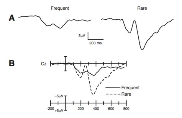
Figure 6.1. Examples of a poor way to plot ERP waveforms (A) and a good way to plot them (B). Negative is plotted upwards.
