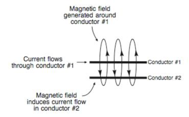
Figure A.1. Relationship between electricity and magnetism. A current is passed through conductor #1, and this generates a magnetic field that circles around conductor #1. As this magnetic field passes through conductor #2, it induces a small current in conductor #2.
