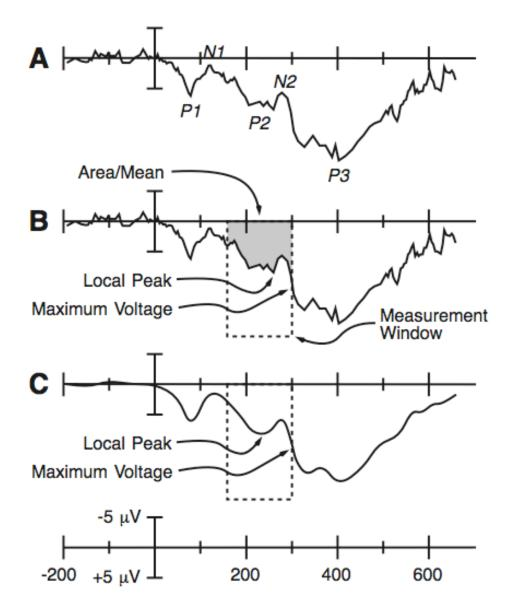
Figure 6.2. (A) ERP waveform with several peaks. (B) ERP waveform, with a measurement window from 150 – 300 ms poststimulus and several measures. (C) Filtered ERP waveform. Negative is plotted upwards.
