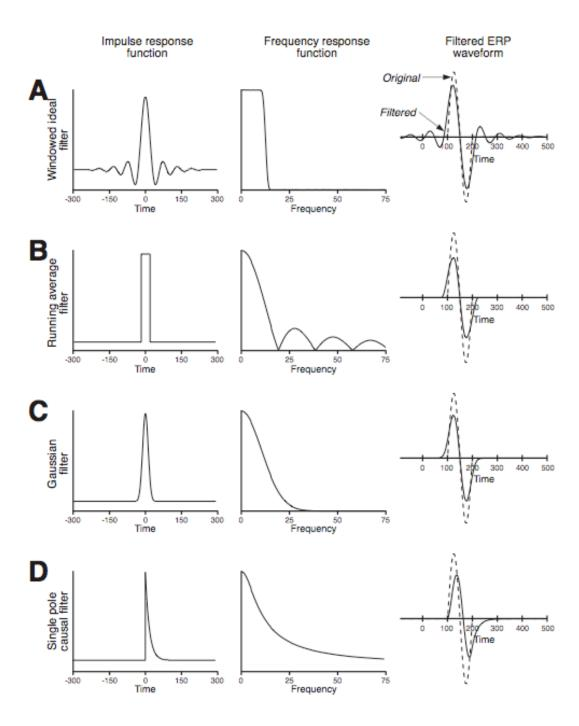
Figure 5.9. Examples of temporal distortions produced by several types of low-pass filters, each with a half-amplitude cutoff of approximately 12.5 Hz. The left and middle columns show the impulse and frequency response functions of the filters, respectively. The right column shows the result of applying each filter to the artificial ERP waveform shown in Figure 5.8A.
