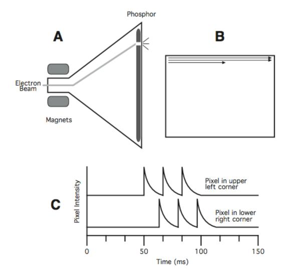
Figure 8.3. Operation of a CRT monitor. (A) The electron beam is directed by a magnetic field to a specific location at the front of the monitor, causing a small spot in the phosphor layer to become illuminated. (B) Raster pattern of the movement of the electron beam over time. (C) Intensity of the luminance from pixels on two different locations on a CRT monitor.
