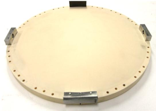
Figure 23: 500 mm diameter POLARBEAR-2 Alumina reimaging lens.
