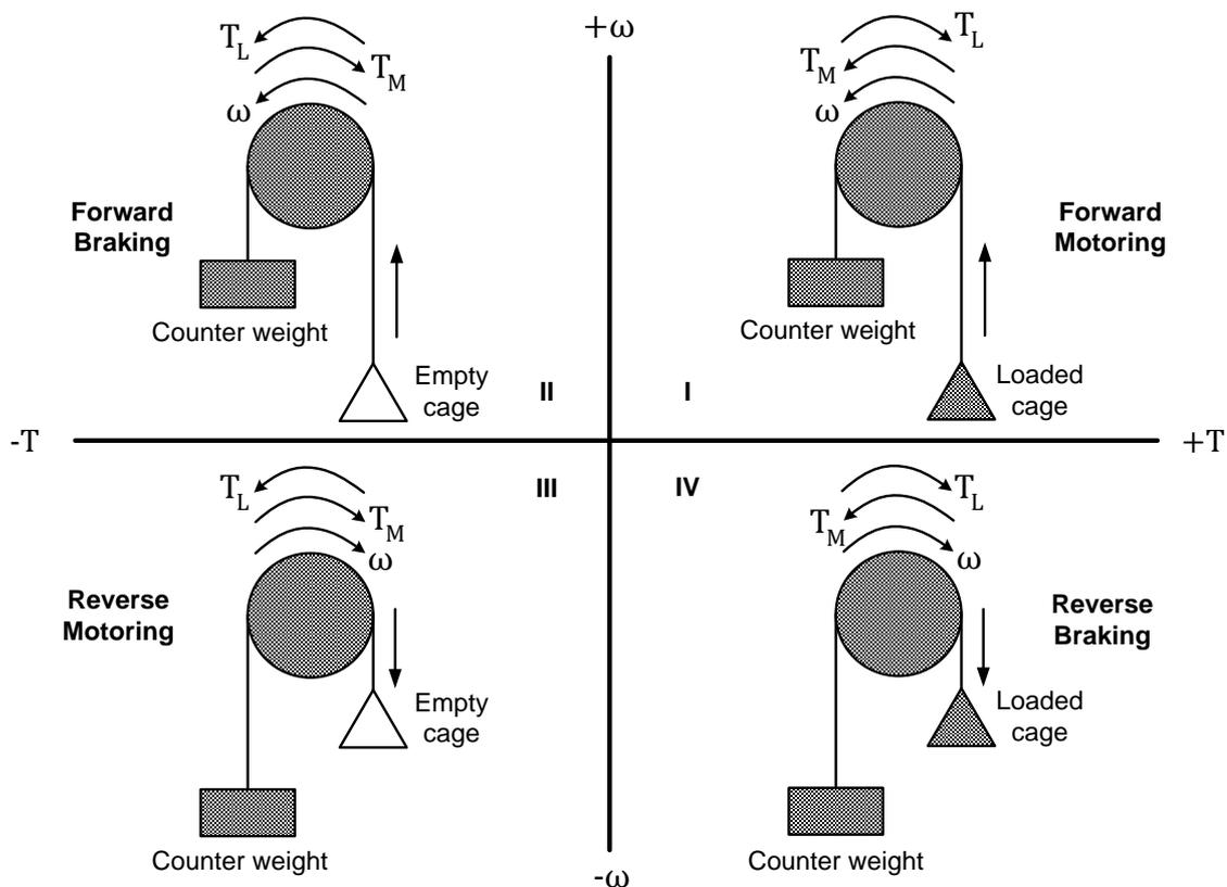
Figure 2.3 Four quadrant operation of a motor driving a hoist load
