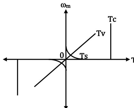
Figure 2 . 7 Friction torque and its components
