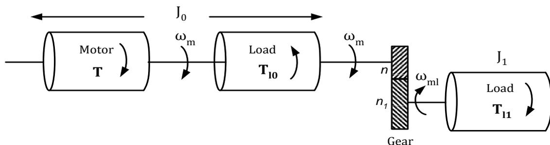
Figure 2.4 Rotational load coupled to motor shaft
