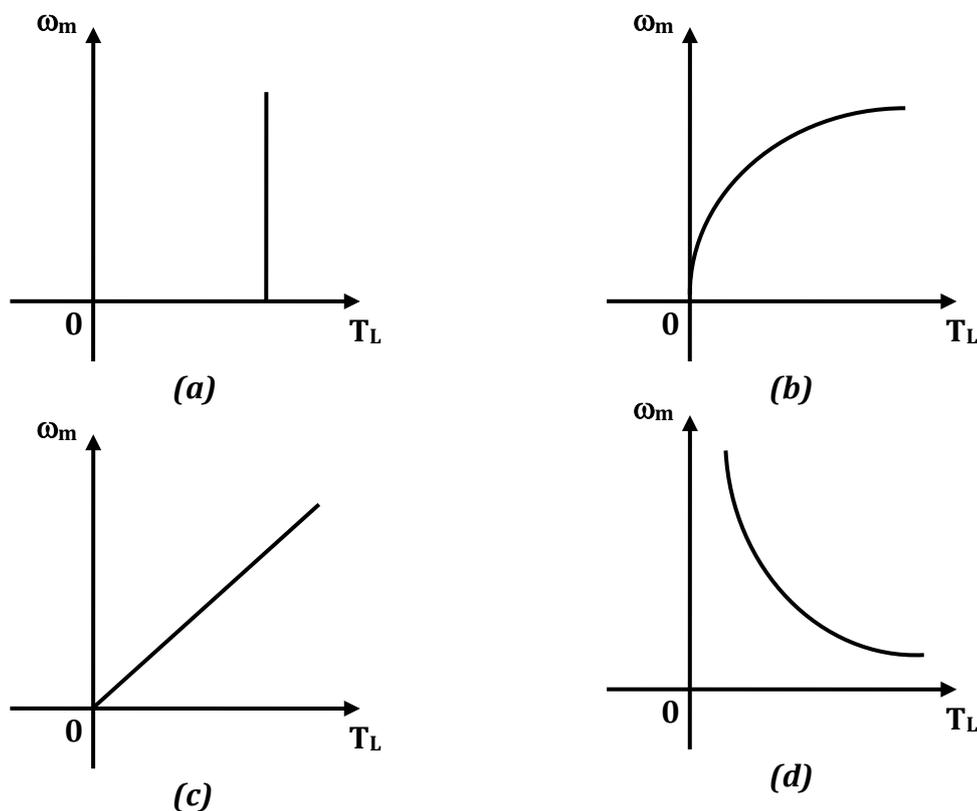
Figure 2.1 Nature of load torque (a)  $T = \text{constant}$  (b)  $T \propto \omega_m^2$  (c)  $T \propto \omega_m$  (d)  $T \propto 1/\omega_m$
