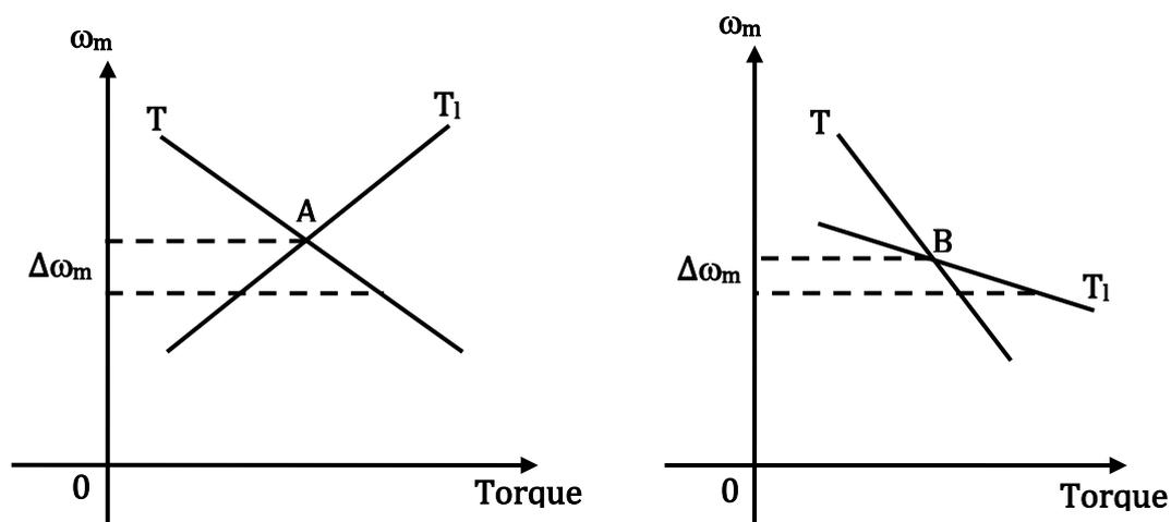
Figure 2.2 Steady state stability: point A-stable, point B-unstable
