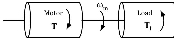
Figure 2.1 Equivalent motor load system
