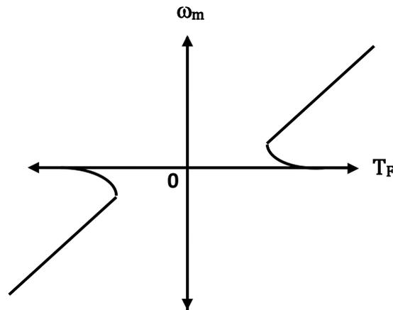
Figure 2 . 6 Variation of friction torque with speed
