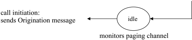
Figure 8.25 IS-95: preparation to set up a call
