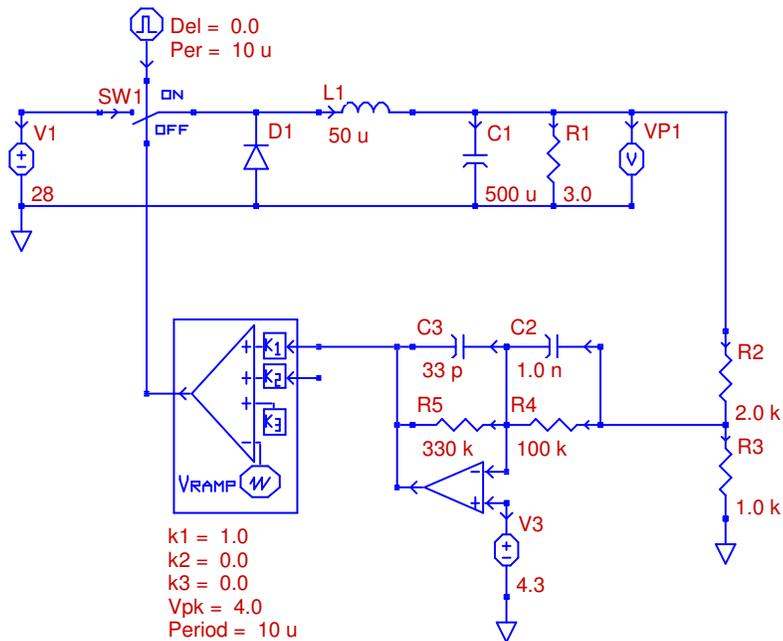
Figure 4.28: PECS Schematic of Lead System
