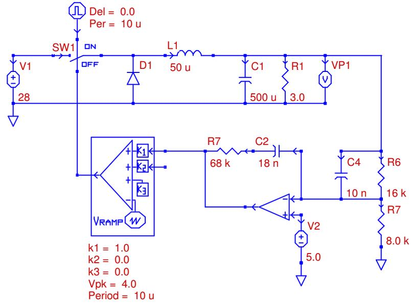
Figure 4.43: PECS Schematic of Extended System
