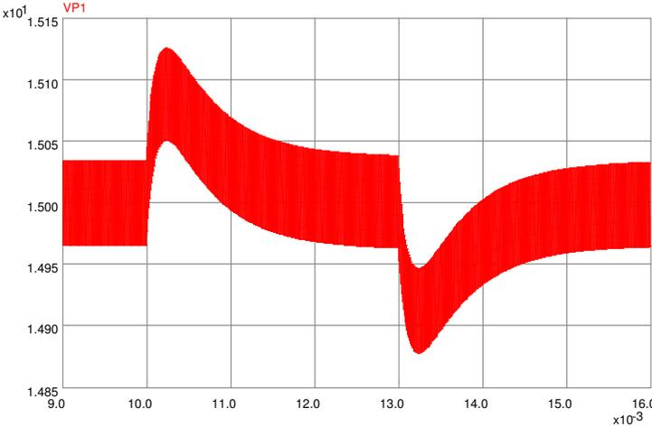
Figure 6.29: PECS Simulation of Voltage Mode Compensated Response to a Supply Voltage Disturbance
