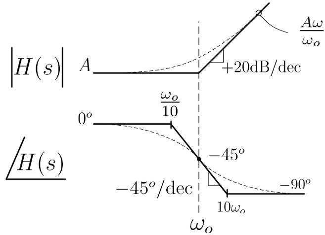
Figure 3.6: Right Half Plane Zero at  $\omega_o$
