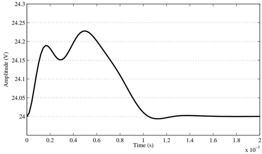
Figure 11.7: Unit step disturbance response of Ćuk converter with ROESFBI compensator.
