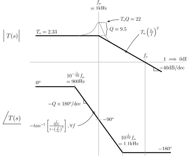
Figure 4.4: Uncompensated Gain and Phase Plot
