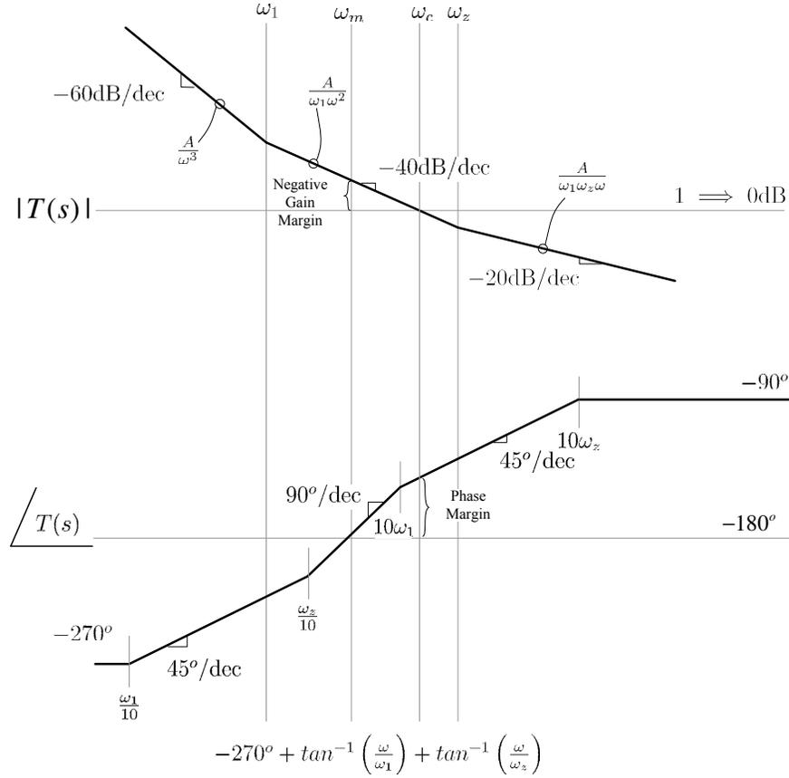
Figure 5.1: Bode Plot: System Loop Gain
