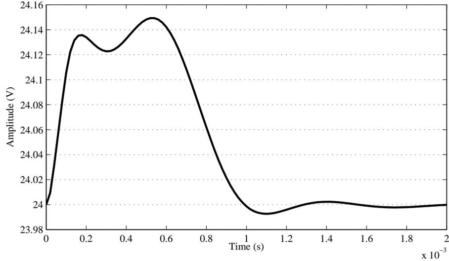
Figure 11.2: Unit step disturbance response of Ćuk converter with ESFBI compensator.
