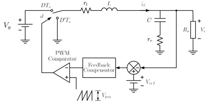
Figure 2.2: Buck Converter Circuit System Diagram
