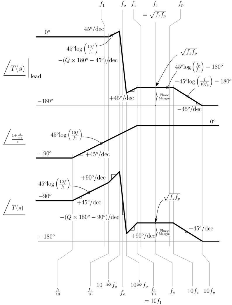
Figure 4.36: Bode Plot of Lead Compensator (150Hz)
