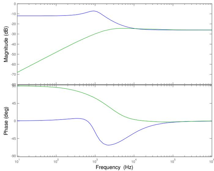
Figure 6.25: MATLAB Bode Plot of  $Z_o$  for Voltage Mode Compensated System
