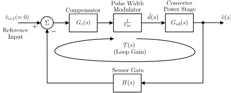
Figure 2.3: Simplified System Diagram
