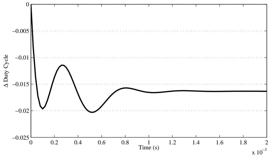
Figure 9.6: Control effort with the full state feedback controller.
