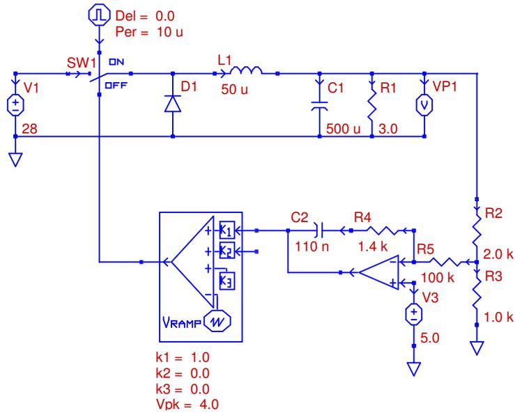
Figure 4.22: PECS Schematic of Dominant Pole with Zero Compensation (10 dB GM)
