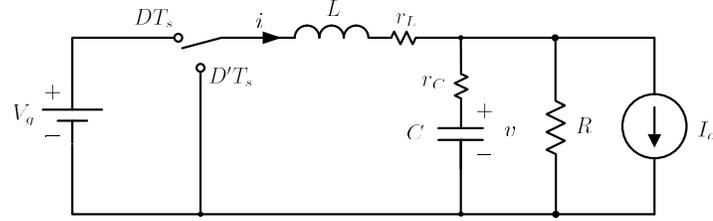
Figure 2.5: Buck Converter Circuit with Non-Ideal Circuit Elements
