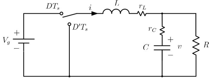
Figure 2.9: Buck Converter Circuit with Non-Ideal Circuit Elements
