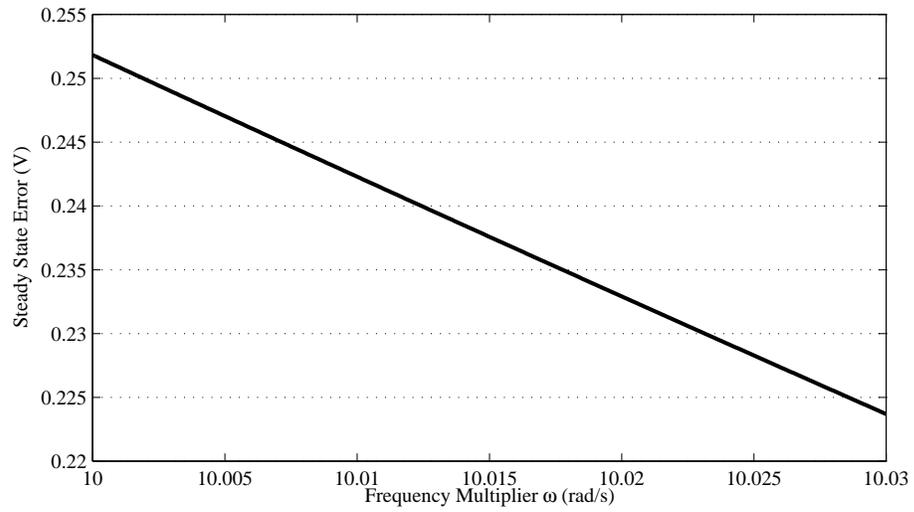
Figure 9.2: Steady state error of unit step disturbance as frequency multiplier is swept.
