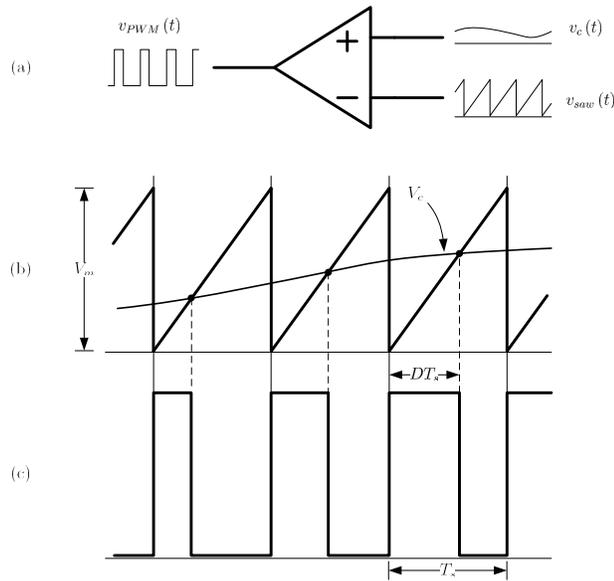
Figure 2.11: PWM Conversion Diagram
