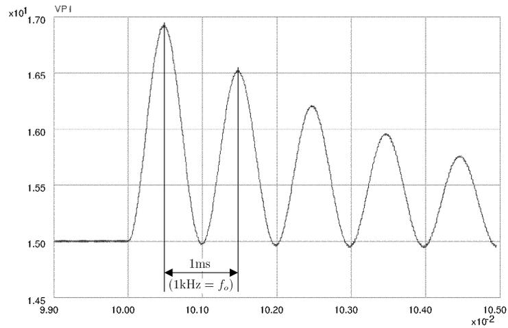
Figure 4.16: Pole of Dominant Pole Simulation Showing Oscillation at Resonant Frequency
