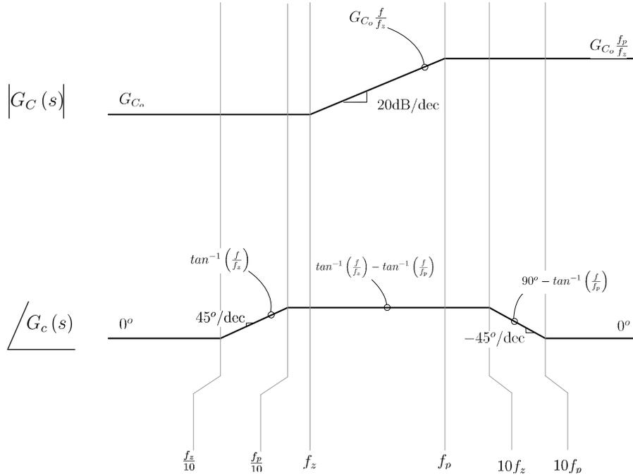
Figure 5.25: Bode Diagram: Lead Compensator
