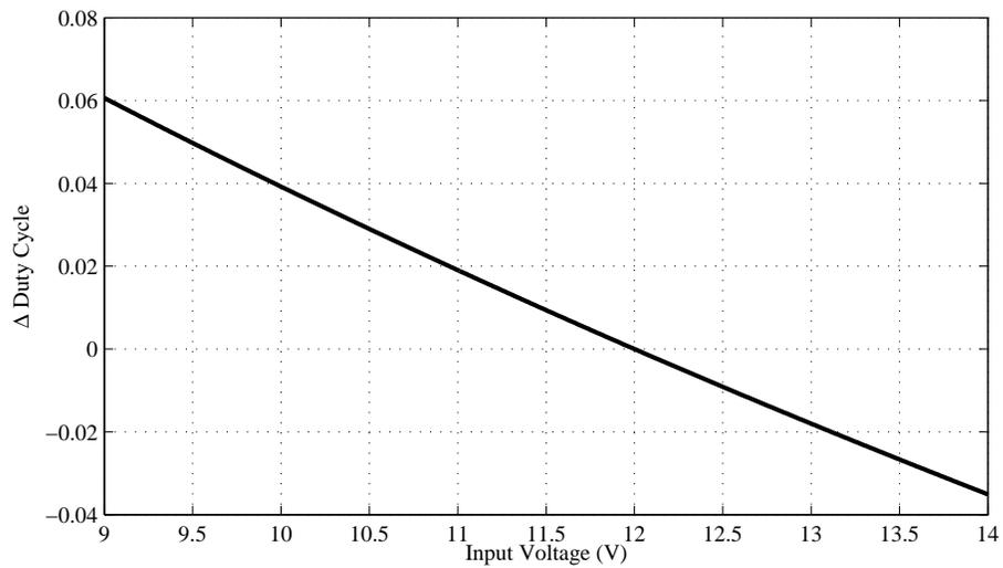
Figure 8.7: The small-signal duty cycle required over the full input voltage range to maintain nominal output voltage.
