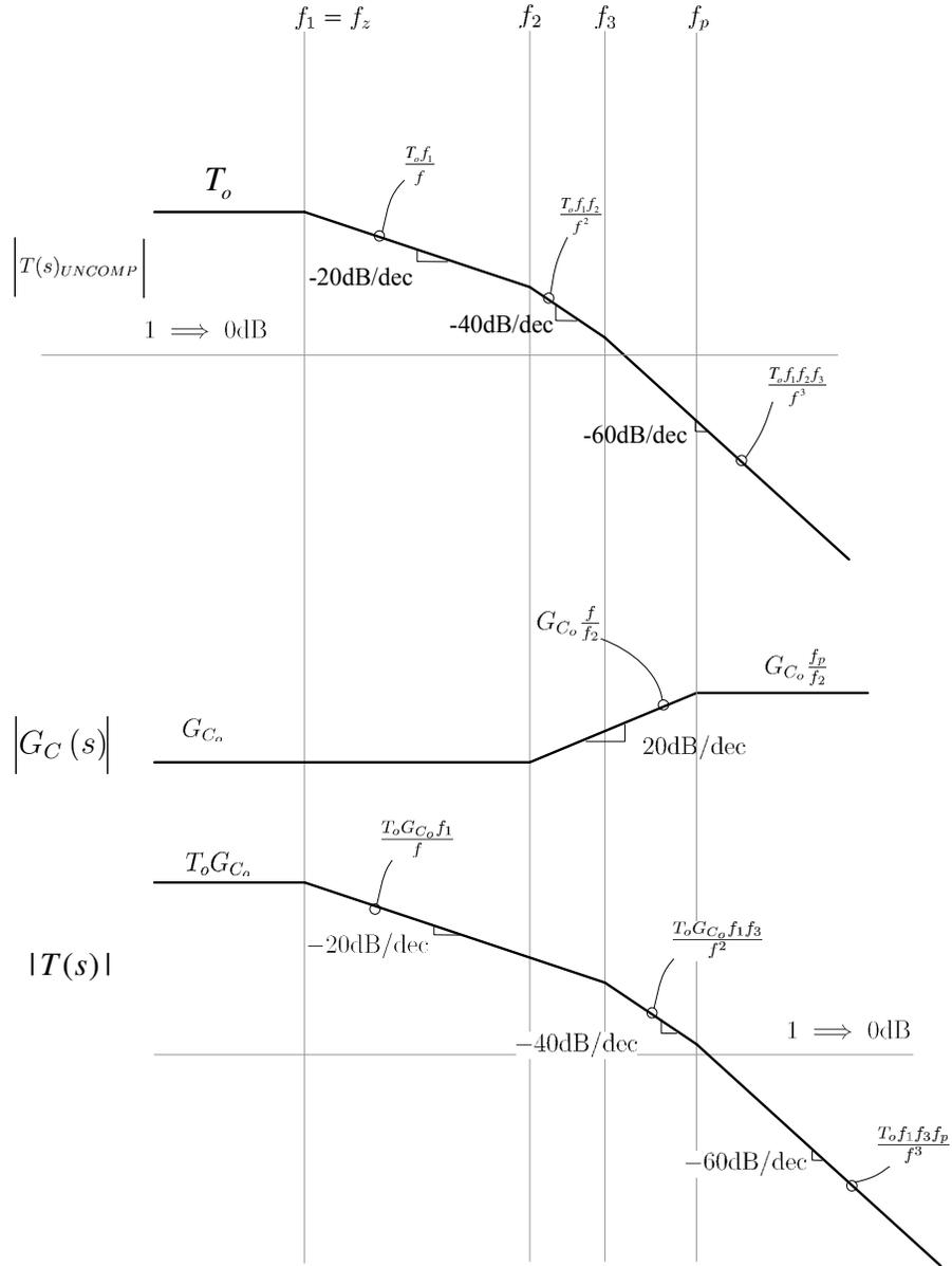
Figure 5.26: Lead Compensation Magnitude Construction
