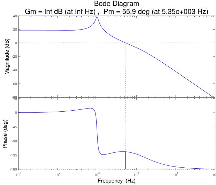
Figure 4.26: Matlab Lead Compensator
