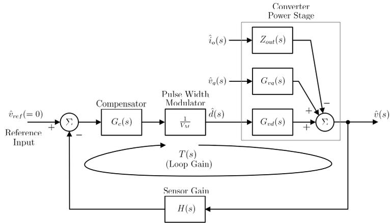
Figure 6.4: Buck converter control loop
