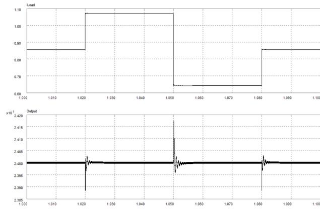
Figure 15.4: Load current disturbance and  $v_o$  response - MRROLQGI/LTR compensator.
