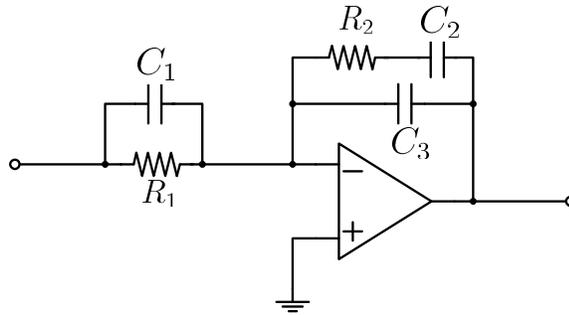
Figure 4.33: Compensator Circuit for Dominant Pole with Lead Compensation
