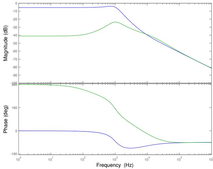
Figure 6.16: MATLAB Bode Plot of  $G_{vg}$  for Active Droop Compensated System
