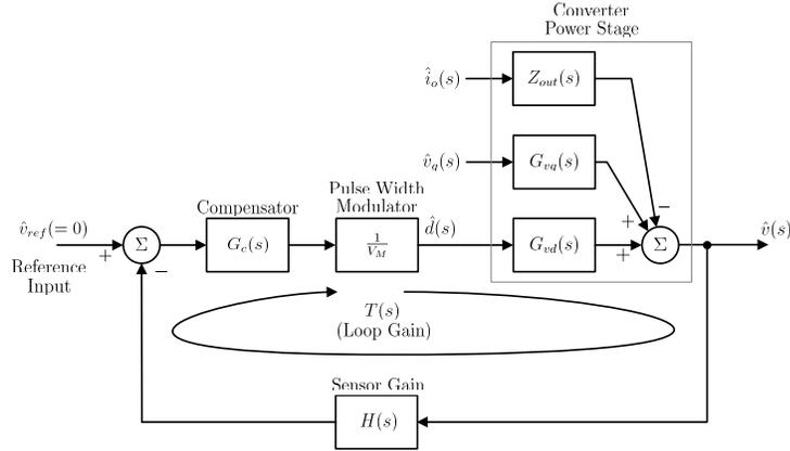
Figure 2.4: Generalized Power System Model
