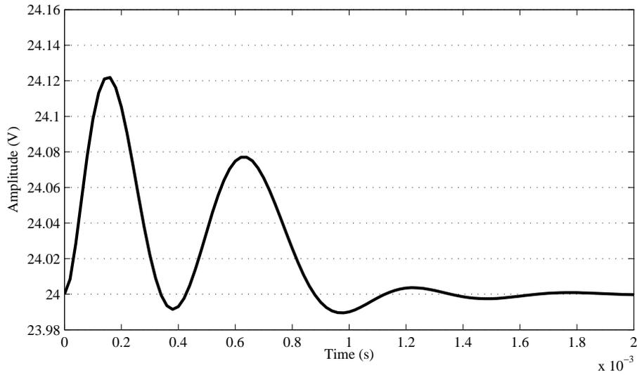
Figure 10.4: Unit step disturbance response of system with FSFBI controller.
