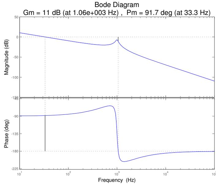
Figure 4.20: Matlab Analysis of Dominant Pole Compensator with Zero
