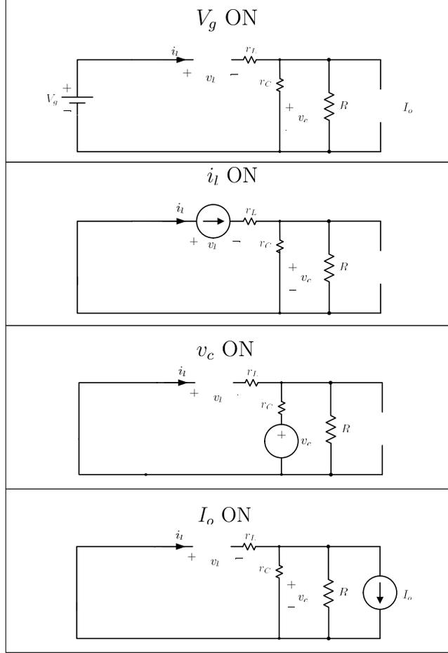
Figure 2.6: Buck Converter Superposition Analysis: DTs
