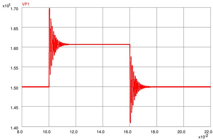
Figure 4.7: PECS Simulation of Open Loop System
