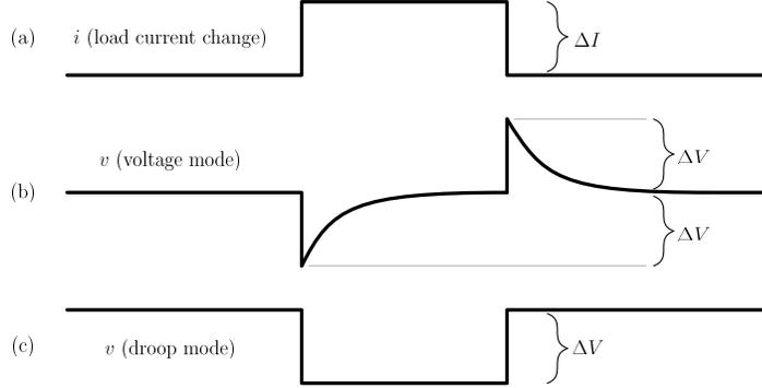
Figure 6.1: Transient Response of System with Droop Control
