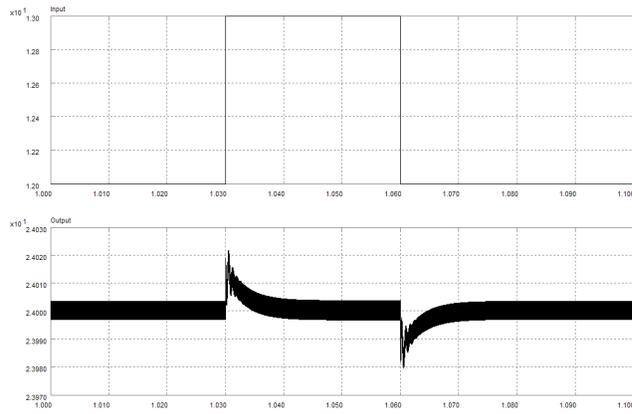
Figure 15.2: Unit step  $v_g$  disturbances and  $v_o$  response - MRROLQGI/LTR compensator.
