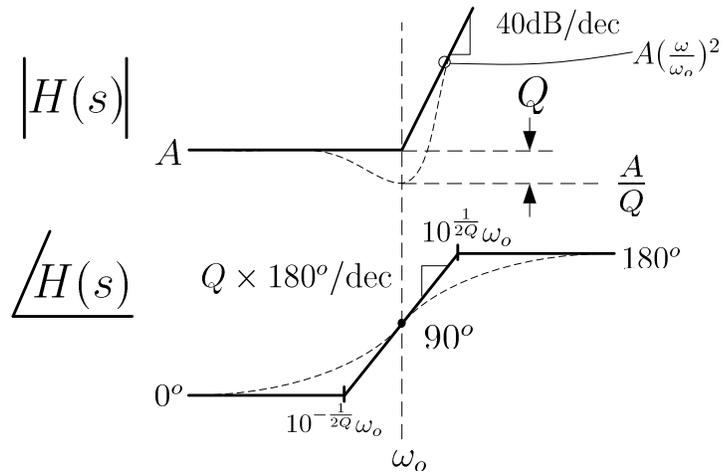
Figure 3.8: Second Order Complex Zero at  $\omega_o$
