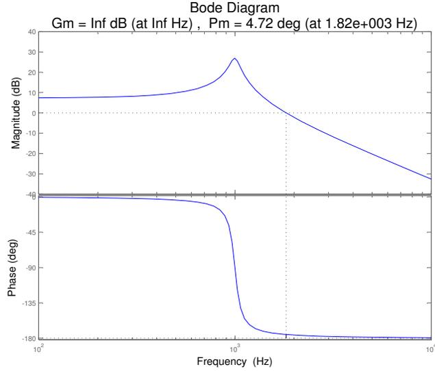
Figure 4.5: Matlab Uncompensated Bode plot
