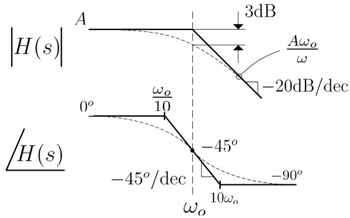
Figure 3.4: Pole at  $\omega_o$
