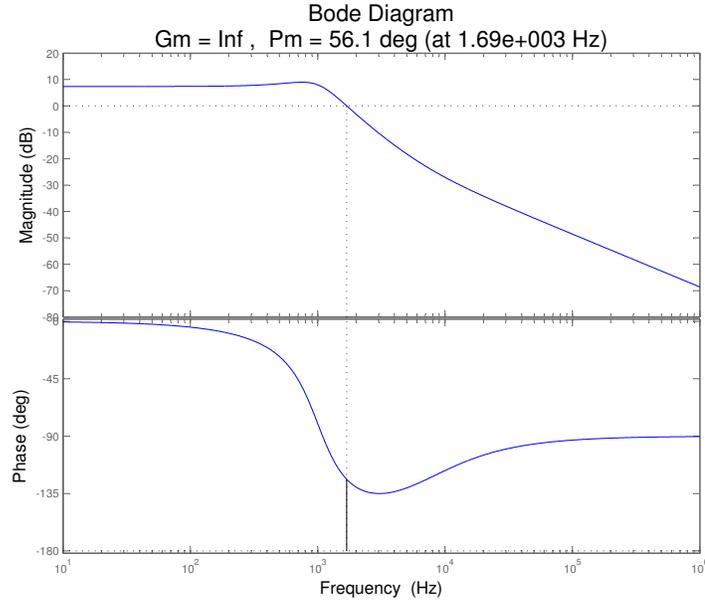
Figure 6.3: MATLAB Uncompensated Bode plot
