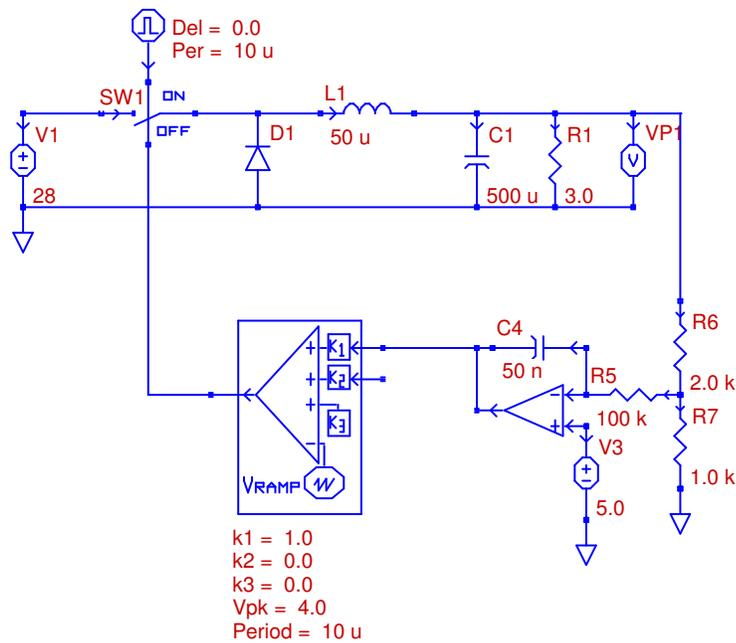
Figure 4.14: PECS Schematic of Dominant Pole Compensated System
