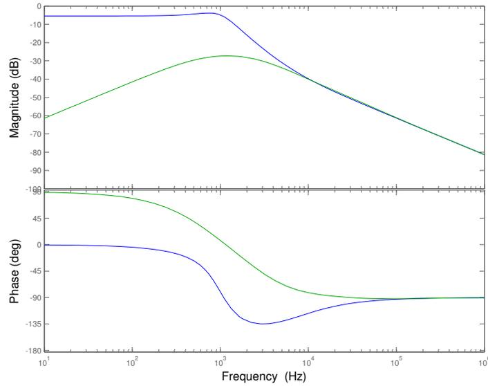
Figure 6.26: MATLAB Bode Plot of  $G_{vg}$  for Voltage Mode Compensated System
