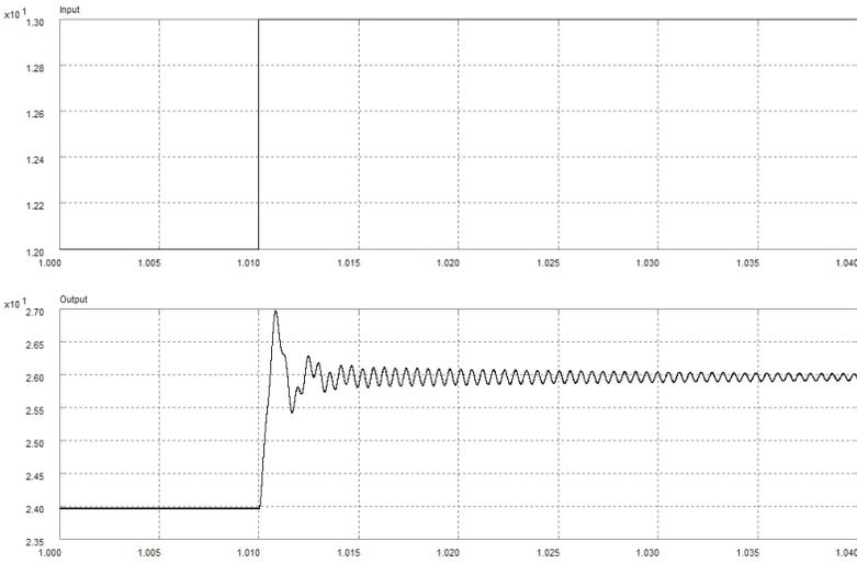
Figure 8.5: Unit step response of the Ćuk converter in PECS.
