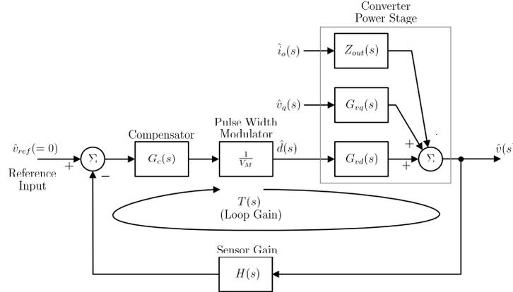
Figure 4.1: Generalized Power System Model
