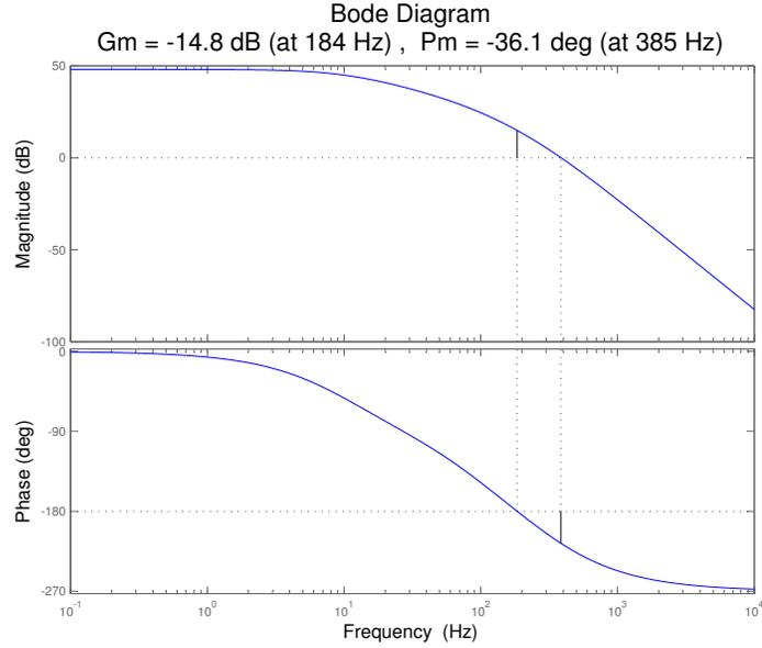
Figure 5.10: Matlab Analysis of Uncompensated System
