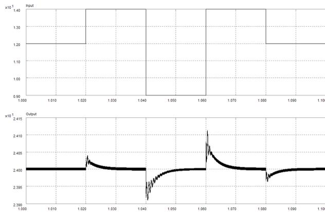
Figure 15.3: Large signal  $v_g$  disturbances and  $v_o$  response - MRROLQGI/LTR compensator.
