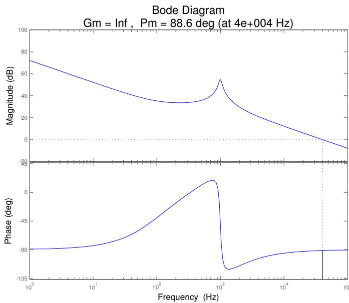
Figure 4.42: Matlab Analysis of Extended Compensator
