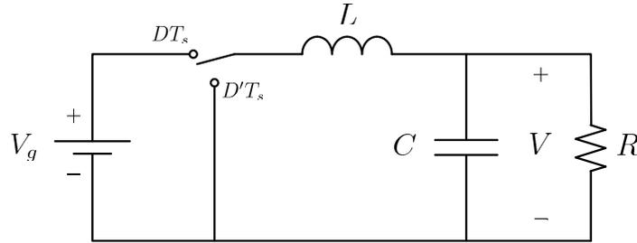
Figure 2.8: Ideal Buck Converter Circuit
