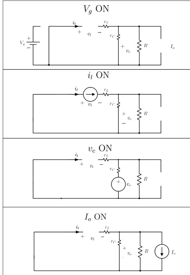
Figure 2.7: Buck Converter Superposition Analysis: D'Ts
