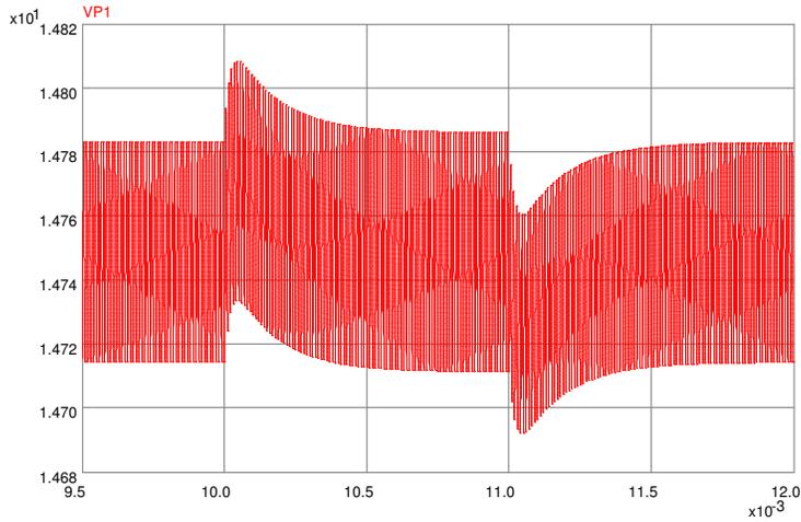
Figure 6.19: PECS Simulation of Active Droop Compensated Response to a Supply Voltage Disturbance
