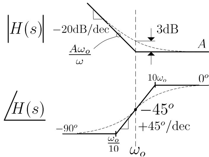
Figure 3.10: Inverted Zero at  $\omega_o$
