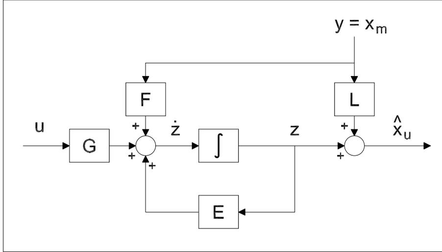
Figure 11.5: Reduced-order estimator construction.
