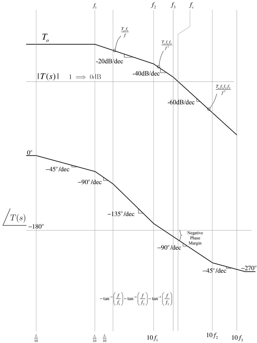
Figure 5.9: Bode Plot: Uncompensated System
