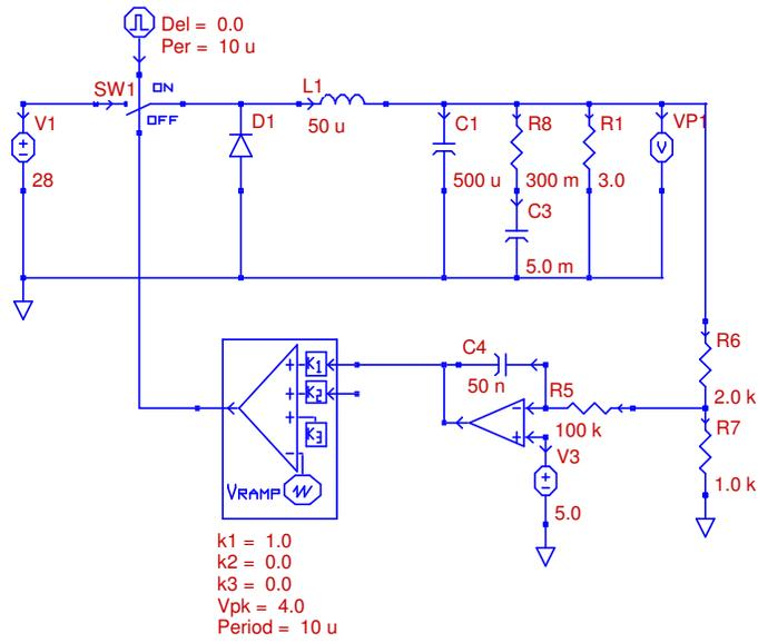
Figure 4.17: PECS Schematic of Dominant Pole with Damping
