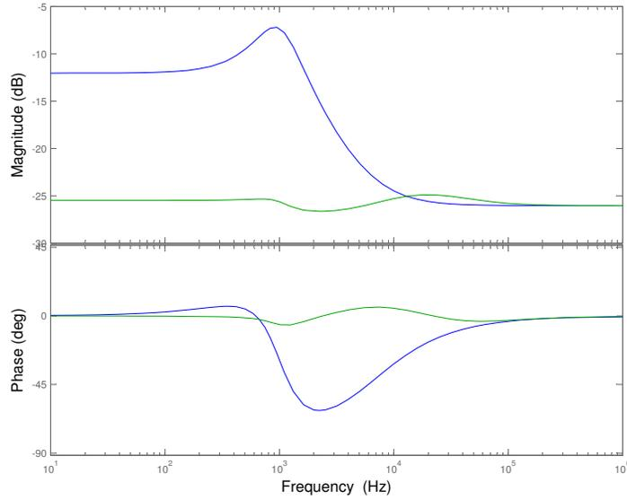
Figure 6.15: MATLAB Bode Plot of  $Z_o$  for Active Droop Compensated System
