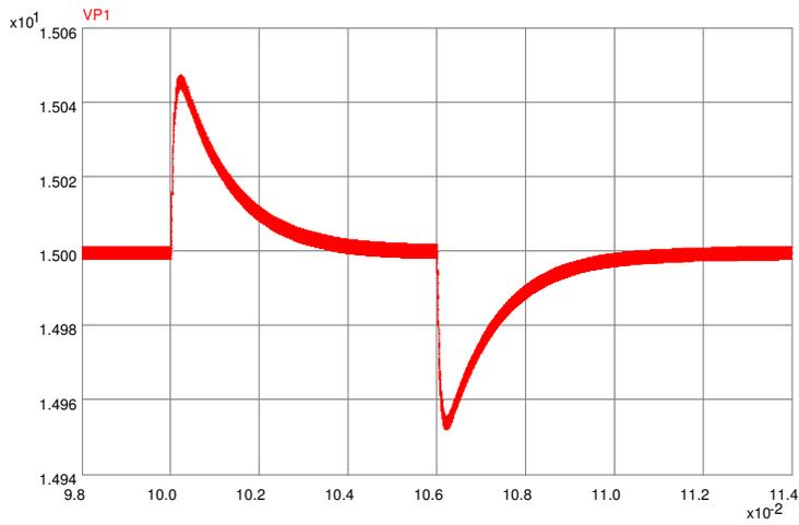
Figure 4.40: PECS Simulation of Lead Compensated System with Zero at 150Hz
