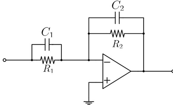
Figure 4.27: op-amp circuit implementation of lead compensator
