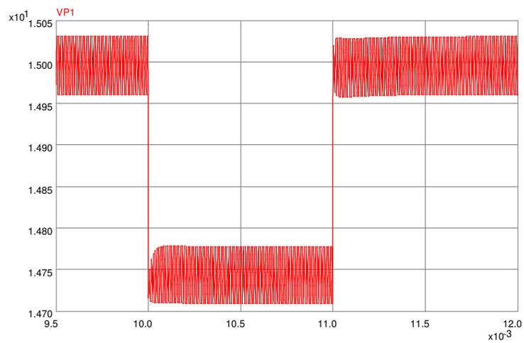
Figure 6.9: PECS Simulation of Passive Droop Compensation Response to a Load Current Step
