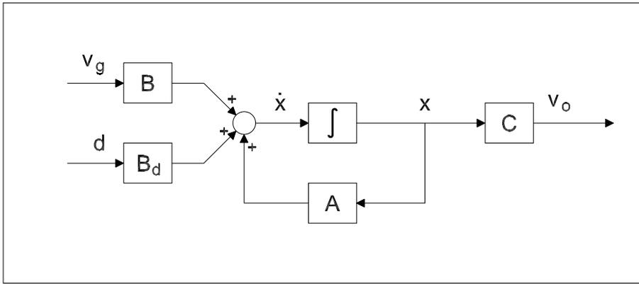
Figure 8.2: State space model of the Ćuk converter.
