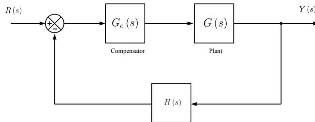
Figure 2.1: Feedback System Block Diagram
