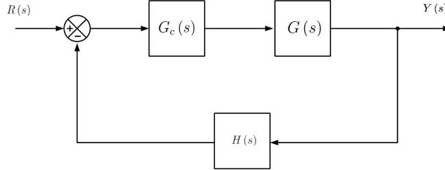
Figure 5.8: Feedback System Block Diagram
