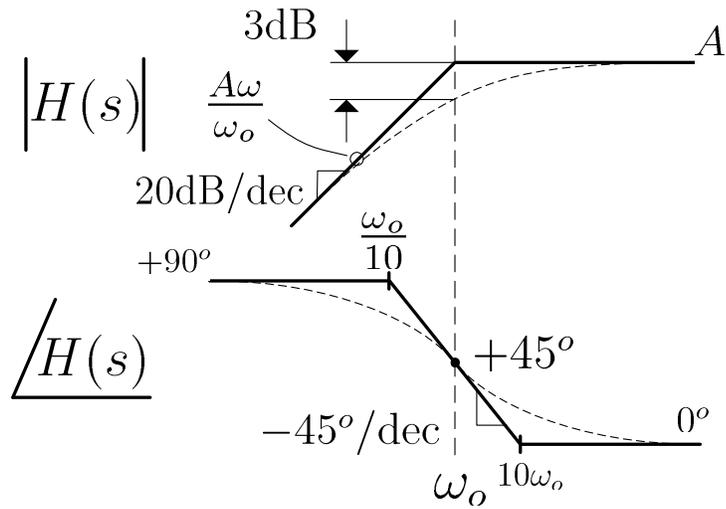
Figure 3.9: Inverted Pole at  $\omega_o$
