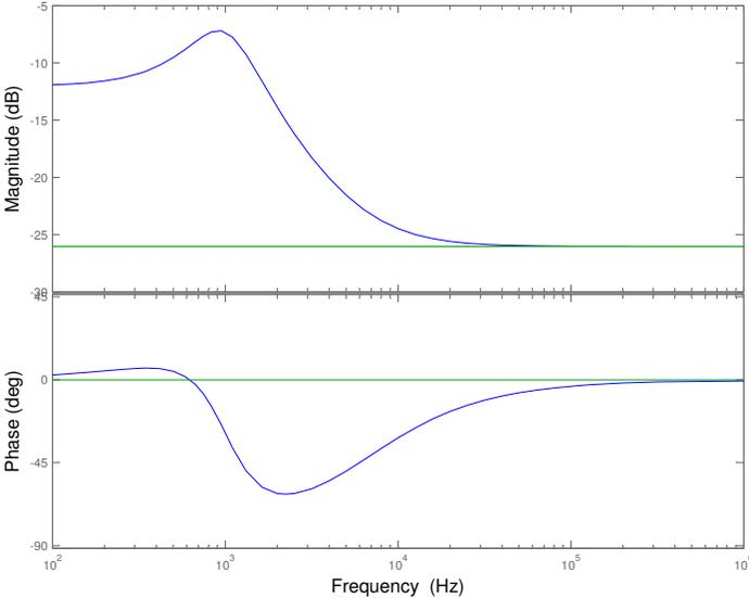
Figure 6.6: MATLAB Bode Plot of  $Z_o$  for Passive Droop Compensated System
