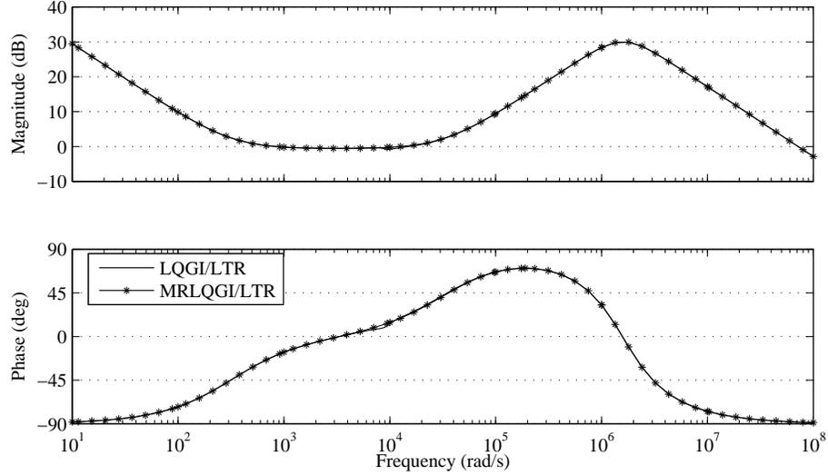
Figure 13.3: Compensator frequency response comparison following model reduction.
