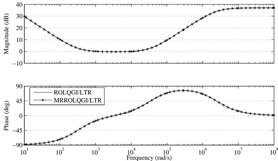
Figure 13.7: Comparison of compensator frequency response - ROLQGI/LTR and MRROLQGI/LTR.
