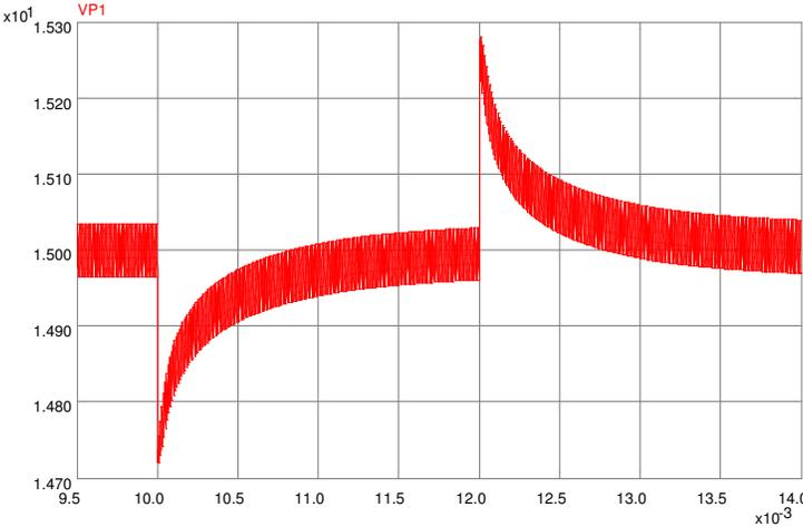
Figure 6.28: PECS Simulation of Voltage Mode Compensated Response to a Load Current Step
