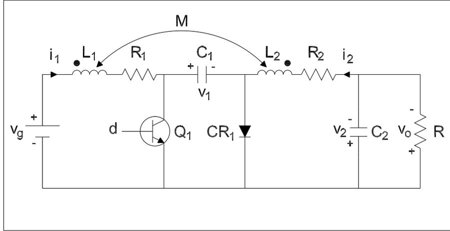
Figure 8.1: Ćuk converter with inductor equivalent series resistances.
