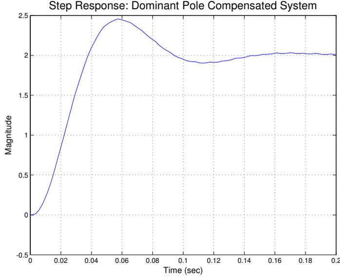
Figure 5.17: Step Response of the Dominant Pole Compensated System
