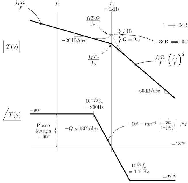
Figure 4.11: Open Loop System Gain and Phase with Dominant Pole Compensation
