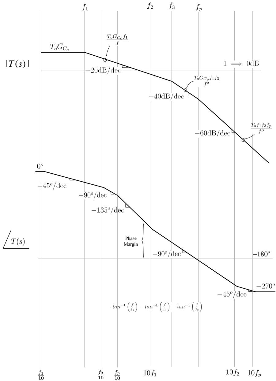
Figure 5.27: Lead Compensated System
