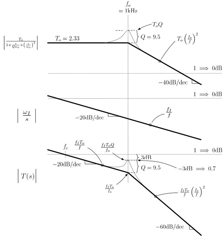
Figure 4.10: Graphical Construction of Gain Asymptotes for Dominant Pole Compensated Open Loop
