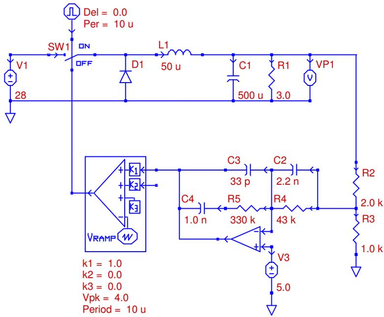
Figure 4.34: PECS Schematic of Lead Compensated System with Zero at 500Hz
