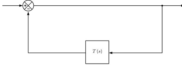
Figure 5.3: Closed-Loop realization of  $T_s$
