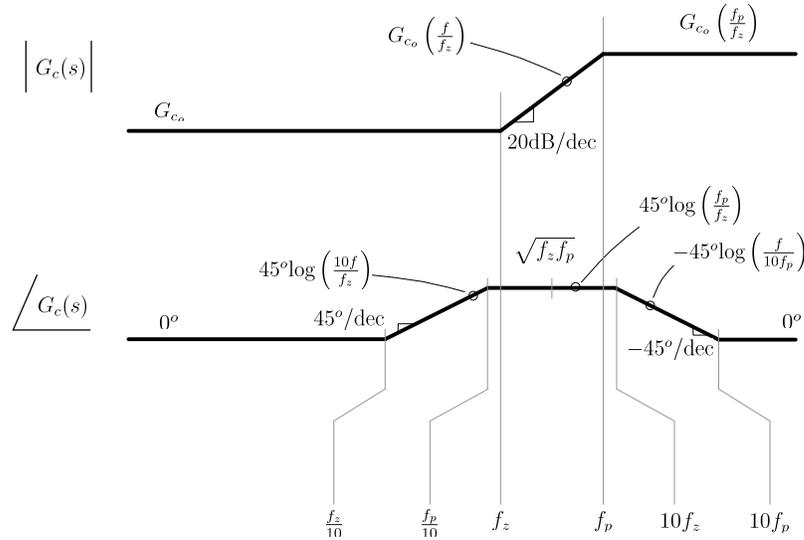
Figure 4.24: Bode Plot of Lead Compensator
