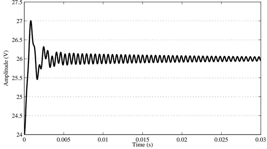
Figure 8.3: Ćuk converter output voltage response to a unit step disturbance in  $v_g$ .
