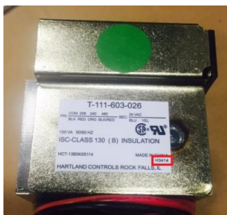
Figure 6 – Identification of transformers certified as conforming are shown below assembled in the electrical box
