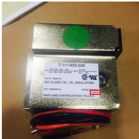
Figure 5 – Transformers reworked by manufacturer and marked with green dot are appropriate for use
