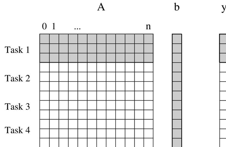
A coarse grained counterpart to the dense matrix-vector product example. Each task in this example corresponds to the computation of three elements of the result vector.
