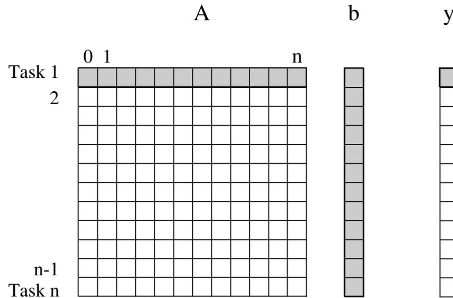
Computation of each element of output vector  $y$  is independent of other elements. Based on this, a dense matrix-vector product can be decomposed into  $n$  tasks. The figure highlights the portion of the matrix and vector accessed by Task 1.
