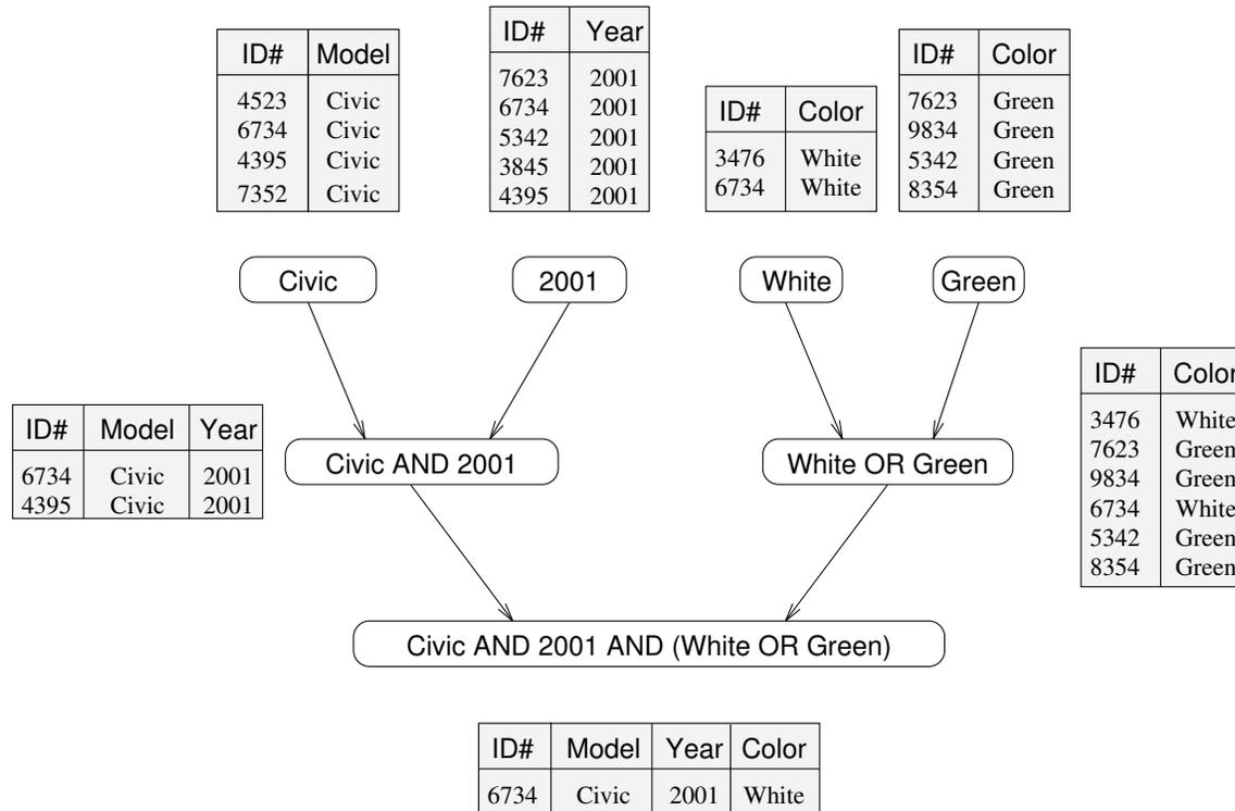
Decomposing the given query into a number of tasks. Edges in this graph denote that the output of one task is needed to accomplish the next.
