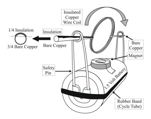
At home electric motors are used in many gadgets – fan, cooler, fridge, mixer, washing machine etc. Modern life would come to a standstill without the electric motor. If you have the materials this simple electric motor can be made in 15-minutes. You will need a new 1.5-volt battery, two long safety pins, a 1-cm wide rubber band from an old cycle tube, 1-meter of 20-gauge (indicated the thickness) insulated copper wire used for motor rewinding and a magnet.
