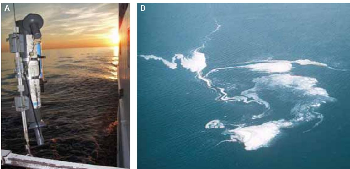
**Figure 2.30** Bottom water sampler (panel A) and free sulphide at the surface of the water in Odense Fjord, released because of hypoxia (panel B).
