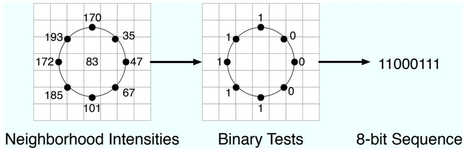
Figure 2: An example of Local Binary Pattern ( $LBP_{8,2}$ ). For a given pixel, the Local Binary Pattern is an 8-bit code obtained by verifying whether the intensity of the pixel is greater or lower than its 8 neighbors.
