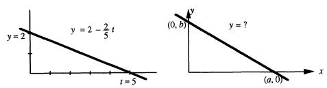
The first line goes down 2 and across 5. The slope is  $\frac{-2}{5} = -.4$ . The minus sign is because y decreases as t increases – the slope of the graph is negative. The "starting point" is y = 2 when t = 0. The equation is y = 2 - .4t. Check that this gives y = 0 when t = 5, so the formula correctly predicts that second point.
