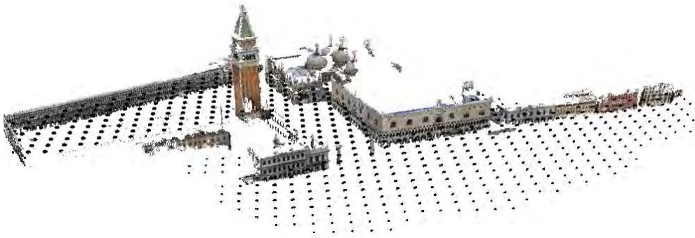
Figure 4.4: Example sampled viewpoints. Camera positions are sampled on the ground plane on a regular 100 \times 100 grid. 24 camera orientations are used for each viewpoint. Cameras not viewing any portion of the 3D model are discarded. This procedure results in about 45,000 valid views for the depicted 3D model.
