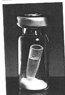
Figure 6.3 Internal hygrostat and heat output due to crystallization of an amorphous phase measured by isothermal microcalorimetry.
