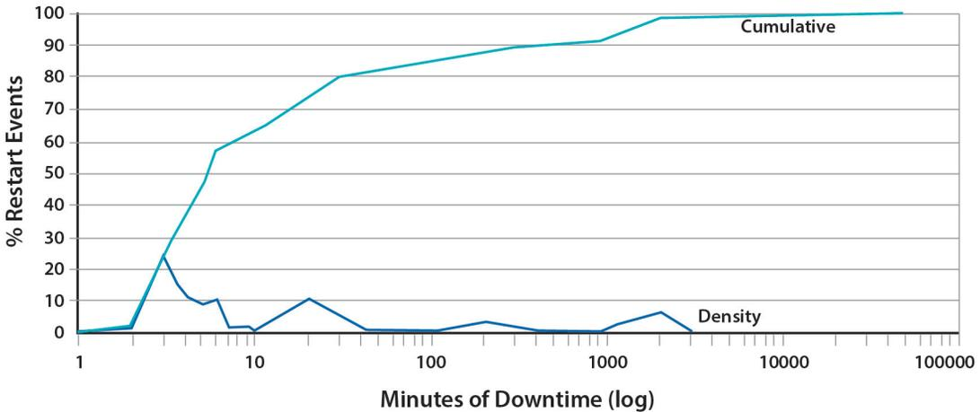
**Figure 7.3:** Distribution of machine downtime, observed at Google over 6 months. The average annualized restart rate across all machines is 4.2, corresponding to a mean time between restarts of just less than 3 months.
