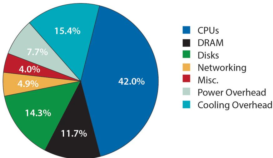
[Figure 1.6](#): Approximate distribution of peak power usage by hardware subsystem in a modern data-center using late 2012 generation servers and a facility energy overhead of 30%. The figure assumes two-socket x86 servers, 16 DIMMs and 8 disk drives per server, and an average utilization of 80%.
