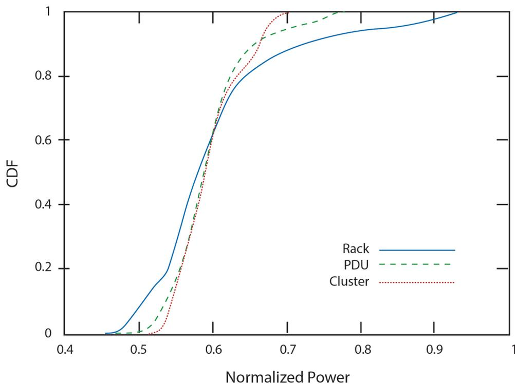
**Figure 5.8:** Cumulative distribution of the time that groups of machines spend at or below a given power level (power level is normalized to the maximum peak aggregate power for the corresponding grouping) (Fan et al. [50]).
