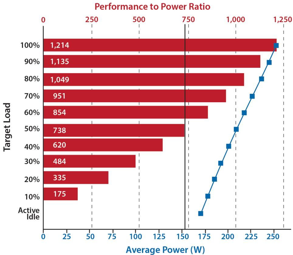
Figure 5.3: An example benchmark result for SPECpower\_ssj2008; energy efficiency is indicated by bars, whereas power consumption is indicated by the line. Both are plotted for a range of utilization levels, with the average metric corresponding to the vertical dark line. The system has a single-chip 2.83 GHz quad-core Intel Xeon processor, 4 GB of DRAM, and one 7.2 k RPM 3.5" SATA disk drive.
