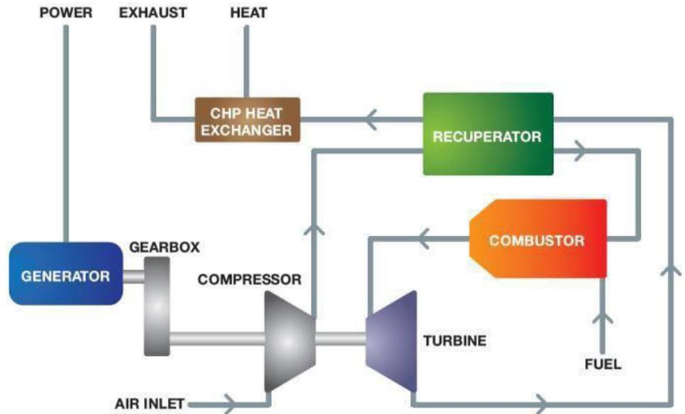
Figure 1. Microturbine configuration for CHP.
