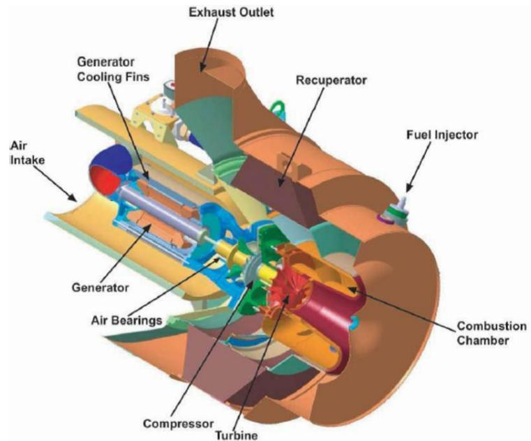
Figure 2. Microturbine illustration.
