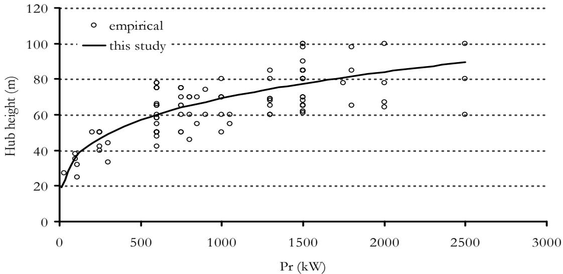
Figure 4: The relation between the rated power of a wind turbine,  $P_r$  (kW) and the hub height (m), as derived from data from existing wind turbines of the German market (Bundesverband WindEnergie, 2001).
