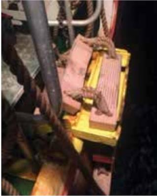
Pilot ladder rigged via an illegal angle bar bracket rather than side rope lashings.
