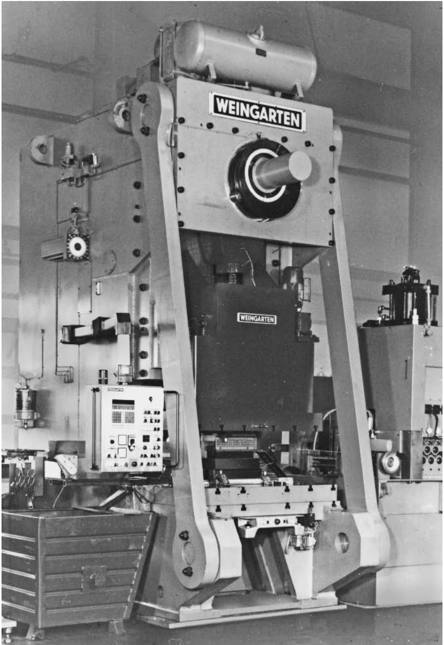
FIGURE 5-12 Open-front power press. Notice the heavy tie rods. (Reprinted with permission from Müller Weingarten AG, Germany.)
