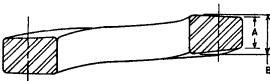
FIGURE 13-22 To prevent worming out, or spreading during tightening, many helical spring lock washers are made so that the peripheral thickness A is less than that at the inner surface B . (Reprinted with permission from H. K. Metalcraft Co., Lodi, NJ.)
