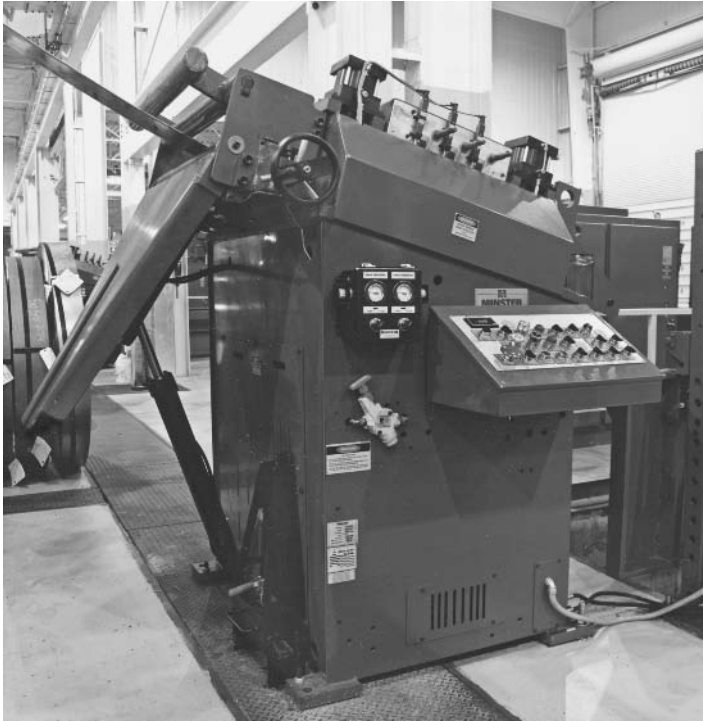
FIGURE 5-23 Straightener with eddy-current drive. ( Reprinted with permission from Minster Machine Co., Ohio. )
