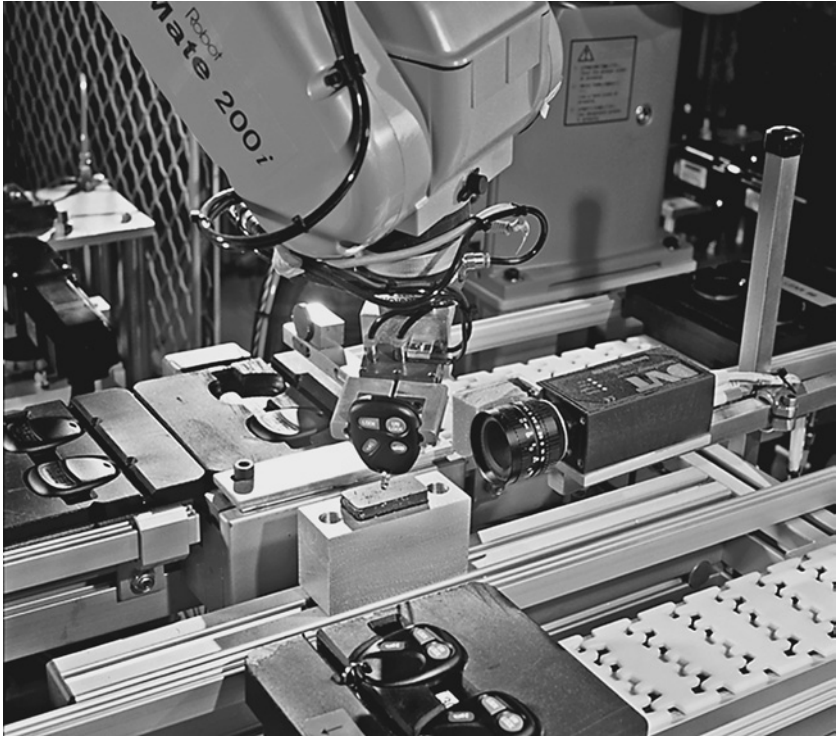
FIGURE 11-6 Camera observing a robotically-inserted component. ( Reprinted with permission from DVT Corporation, Norcross, GA. )
