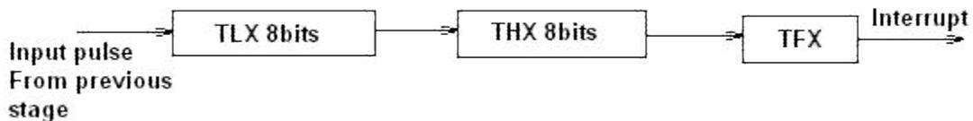
Fig 4.19 Operation of Timer in Mode 1
