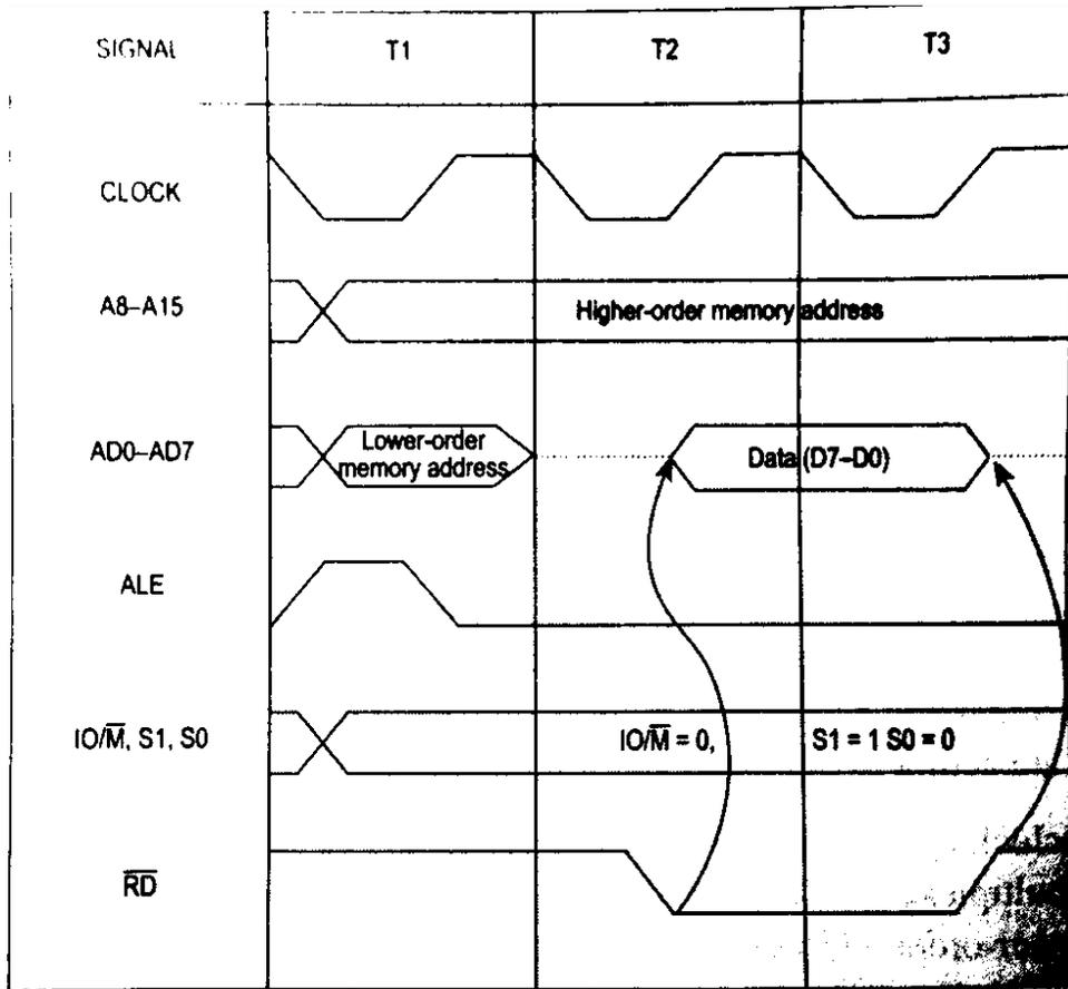
Fig. 8 Timing diagram for memory read machine cycle
