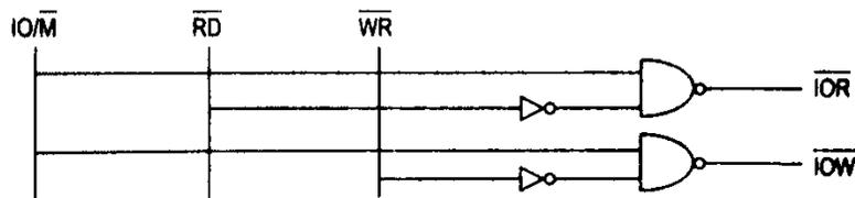
Fig. 20 Generation of  $\overline{IOR}$  and  $\overline{IOW}$  signals
