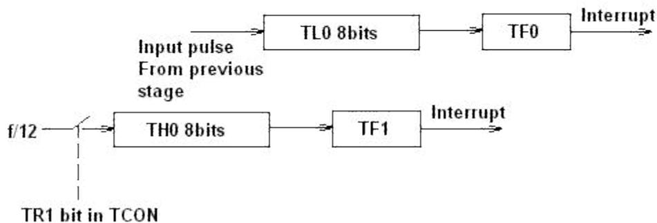
Fig 4.21 Operation of Timer in Mode 3
