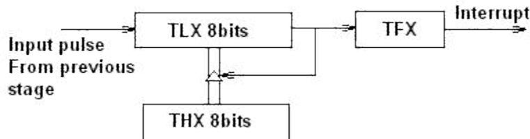
Fig 4.20 Operation of Timer in Mode 2
