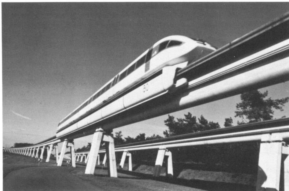
Figure 20.6. Maglev train being tested at the Emsland (Germany) Test Facility. (Photo courtesy of Transrapid International.)
