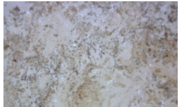
Fig. 11 Surface conditon with industrial contaminant
