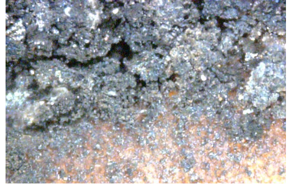
Fig. 10 Surface conditon with NH 4 Cl contaminant
