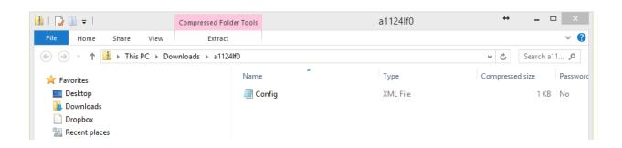
Save this file to an alternate location, such as the desktop. One minor change will need to be made to the file before it can be copied onto the Mesa. Open the config file using a simple text editor (such as notepad), and adjust the URL by removing the "s" in "https".
