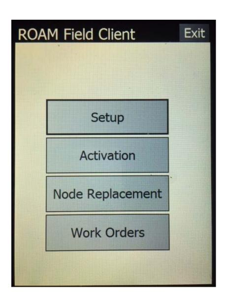
From the Setup menu, first verify that the Mesa has a proper internet connection. To ensure the Mesa can connection to the ROAM server, select the "Test Web Server" button. If the Mesa has a connection to the ROAM server, a notification will pop up saying "The server responded".
