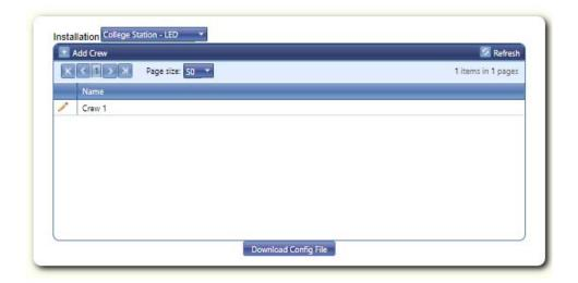
After the crew has been set up, the config file can then be downloaded from the portal. From the same tab, click the "Download Config File". A compressed folder will download, the contents of which will have a "config.xml" file.
