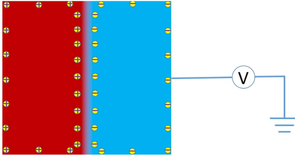
Figure 5. Designed schematic diagram of experimental setup for confirming Yuheng Zhang effect. Shock waves penetrate the metal sample from left to right. The red area denotes compressed zone after shock waves whereas the blue area is uncompressed zone in front of shock waves. The yellow circled with “+” and “-” signs denote the accumulated positive charge and negative electrons, respectively. A time-resolved voltmeter is connected with the zero potential and the blue area.
