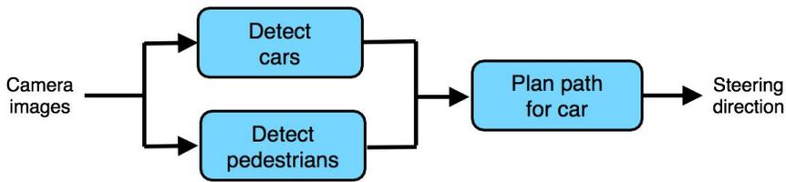
By using this pipeline, you are telling the algorithm that there are 3 key steps to driving: (1) Detect other cars, (2) Detect pedestrians, and (3) Plan a path for your car. Further, each of these is a relatively simpler function--and can thus be learned with less data--than the purely end-to-end approach.
