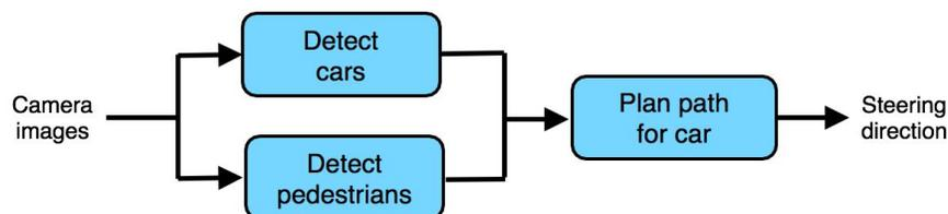
It has three components: One detects other cars using the camera images; one detects pedestrians; then a final component plans a path for our own car that avoids the cars and pedestrians.
