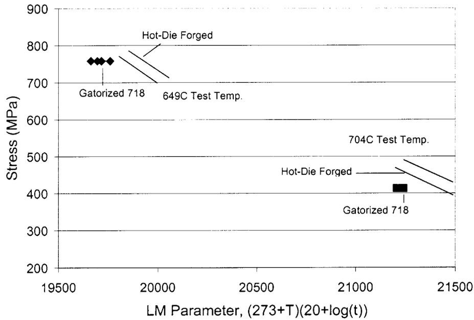
Figure 11 – Combination stress-rupture lives of Gatorized 718 relative to hot-die forged material.
