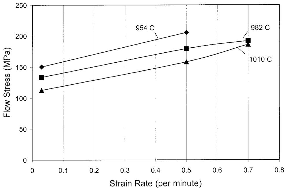
Figure 2 – Flow stresses of the fine-grained billet at several strain rates and temperatures.
