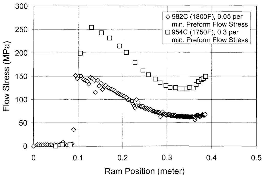
Figure 3 – Flow stresses with ram position in the initial pancake forging (shown for two forging conditions).
