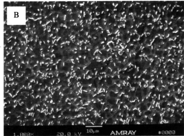
Figure 7 - Example of as-forged microstructure: (A) Optical image, and (B) SEM (Scanning Electron Microscope) image showing delta distribution.
