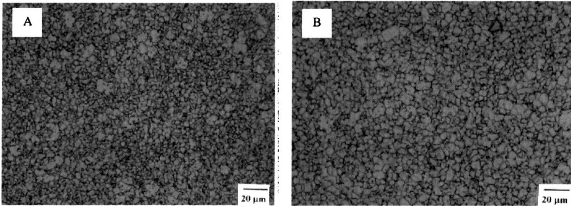
Figure 4: The microstructure following initial pancake forging shown for two forging conditions: (A) 954°C, 0.3 per min. strain rate, (B) 982°C, 0.05 per min. strain rate.
