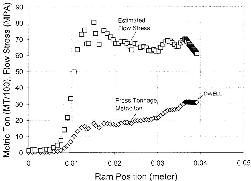
Figure 5 - Example of press tonnage and calculated flow stress in the 2<sup>nd</sup> step contoured forging.
