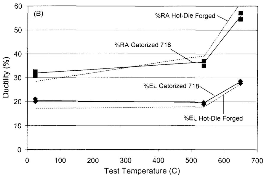
Figure 10– The % elongation and reduction of area of Gatorized 718 relative to hot-die forged material.
