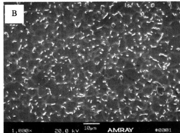
Figure 8 - Example of heat-treated microstructure: (A) Optical image, and (B) SEM (Scanning Electron Microscope) image showing delta distribution.
