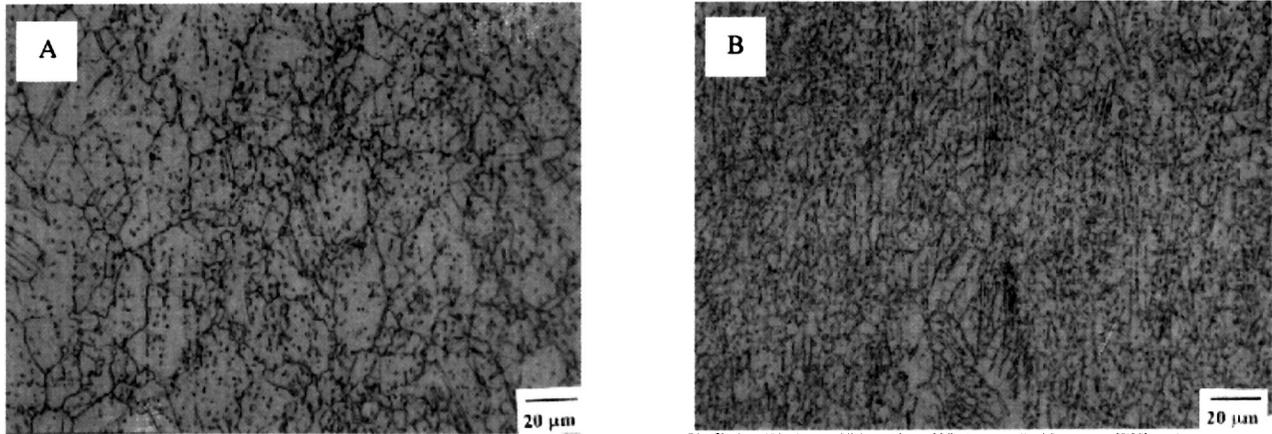
Figure 1 – As-received microstructure of fine-grained billet: (A) Billet center location, and (B) Billet edge location.
