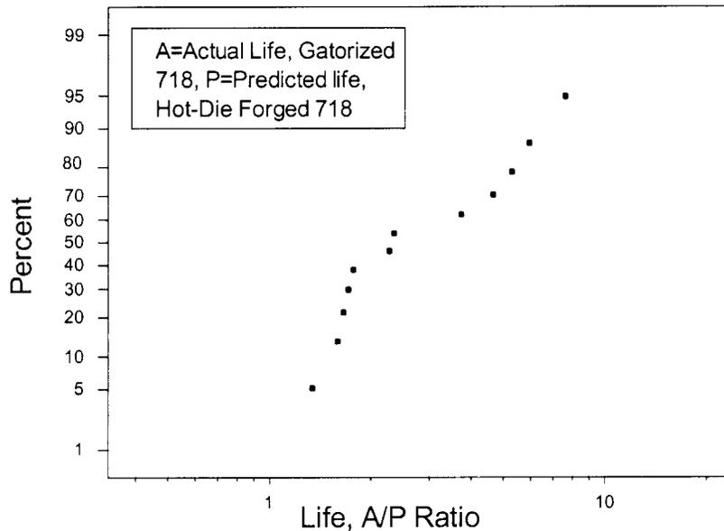
Figure 12 – The notched ( $K_t=2.55$ ) low cycle fatigue life of Gatorized 718 relative to hot-die forged material.
