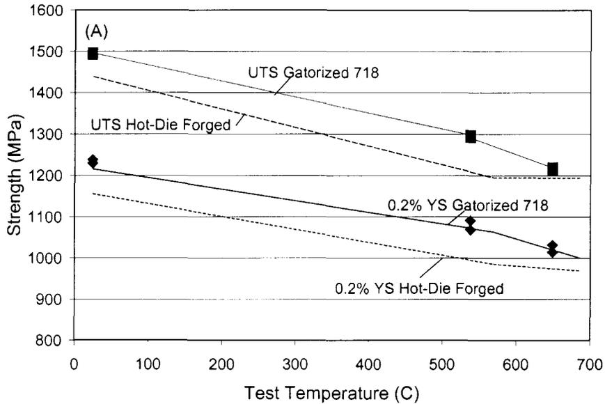
Figure 9 – The 0.2% yield strength and ultimate tensile strength of Gatorized 718 relative to hot-die forged material.
