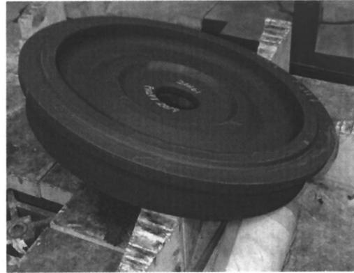
Figure 6 - Illustration of contoured forging (approximate size: 60 cm in diameter).
