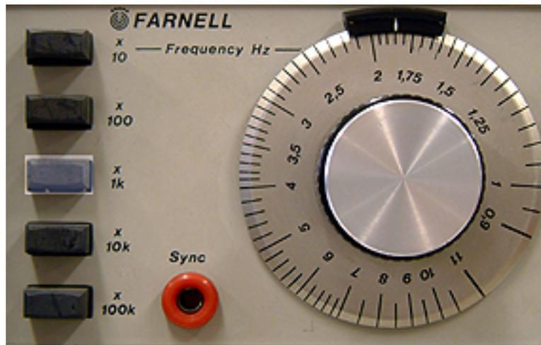
In this example the x 1k button is depressed denoting that all the values on the dial should be multiplied by 1000. The dial is reading 1.85 which means the frequency is set to 1850Hz or 1.85kHz
