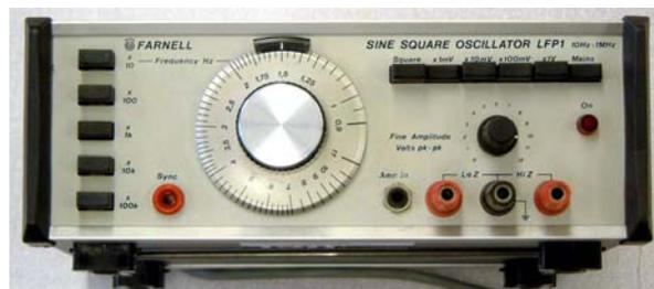
To set the frequency first select the appropriate range using the buttons and then use the large knob to set the exact frequency (note that the scale on this varies as you go round the dial).
