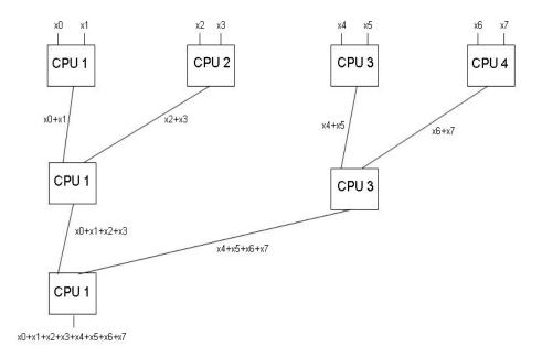
Figure 2: Adding 8 numbers on 4 Parallel Processors
