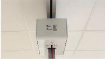
Place the hoist at the yellow marking approx. 1 meter from the end of the traverse rail and Combi Lock.
