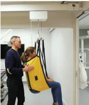
When the Combi Lock has engaged position yourself behind the patient and push lengthwise the traverse rail through the Combi Lock. The patient is still facing / looking lengthwise the traverse rail.
