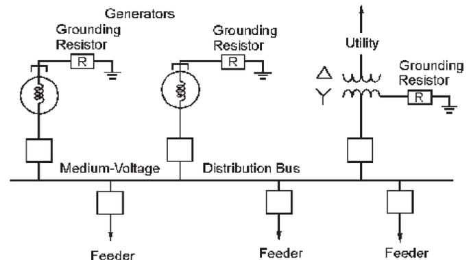
Fig. 1. Medium-voltage industrial distribution system with multiple sources.
