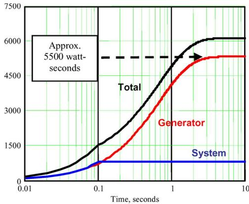
Fig. 3. Watt-second fault energy versus time.
