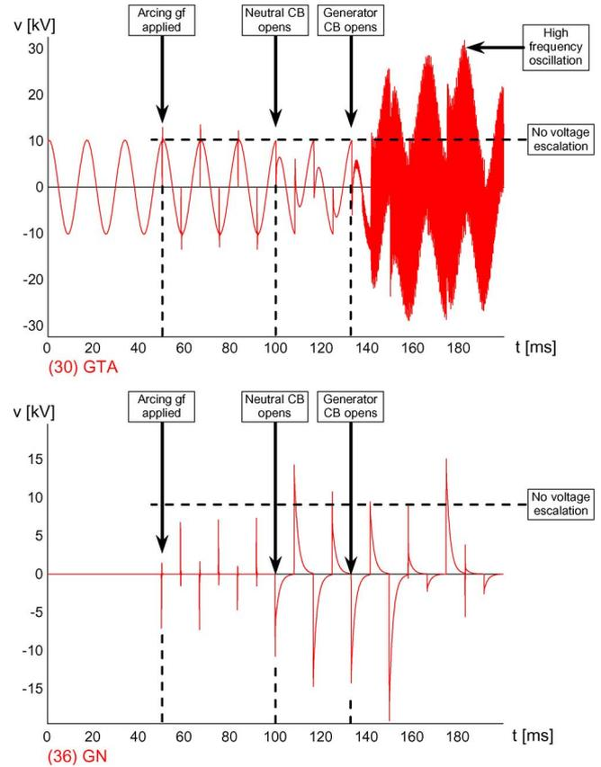
Fig. 13. Generator terminal voltage (top) and neutral voltage (bottom) for Case 7b with HRG component and arcing ground fault at 50 ms and internal voltage decay ( $T_{1g}$  of 1.0).
