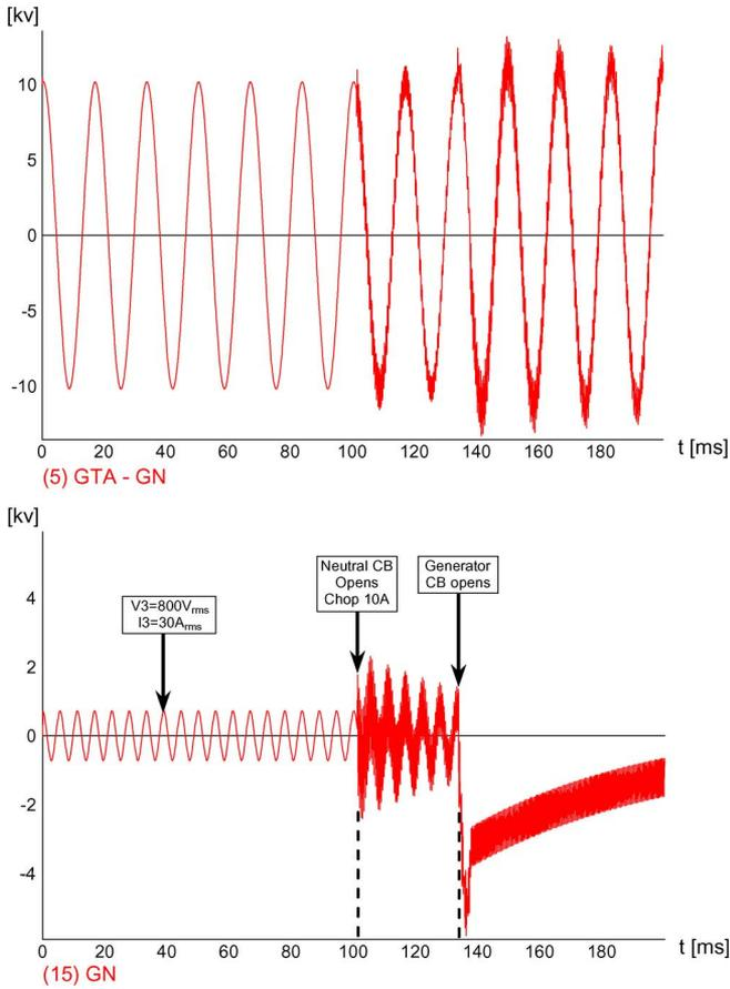
Fig. 10. Generator terminal voltage (top) and neutral voltage (bottom) for Case 4 - Neutral breaker opens in three cycles, and the main breaker opens in five cycles (chop at 10 A of third harmonic current).
