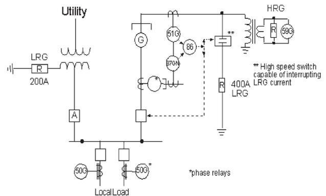
Fig. 5. Hybrid grounded and associated ground fault protection.
