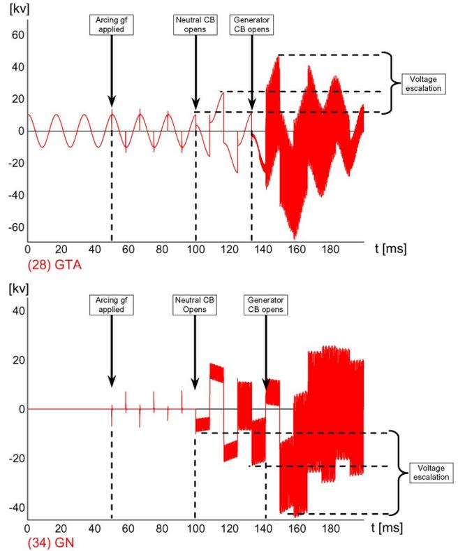
Fig. 11. Generator terminal voltage (top) and neutral voltage (bottom) for Case 6-generator ungrounded - Neutral breaker opens in three cycles, and the main breaker opens in five cycles (arc ground fault on phase-A).
