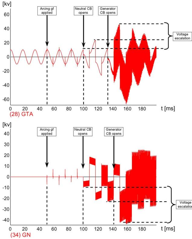
Fig. 12. Generator terminal voltage (top) and neutral voltage (bottom) for Case 6b (generator ungrounded) arcing ground fault at 50 ms and internal voltage decay ( $T_{1g}$  of 1.0).
