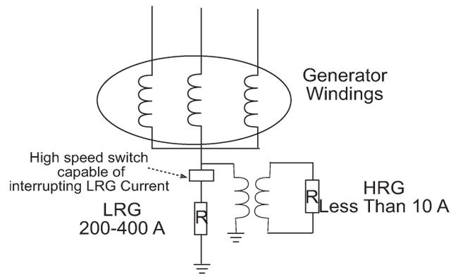
Fig. 4. Generator hybrid ground.
