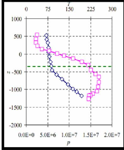
**Figure 3.** PT static profile "Wells-A" before stimulation (failed attempt)
