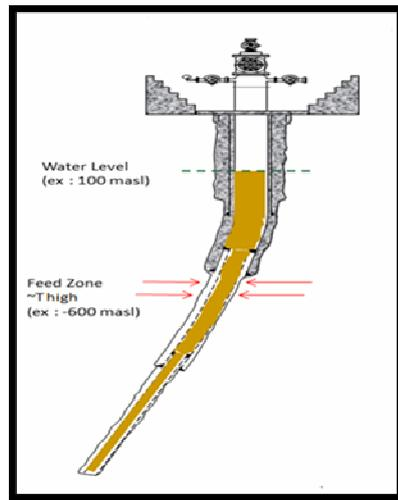
**Figure 1.** Initial condition of non-artesian geothermal wells
