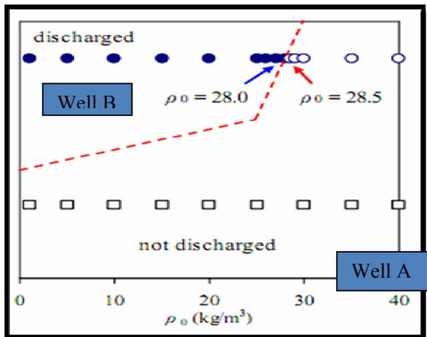
**Figure 5.** Flow occurrence as function of  $\rho$  for the two wells [1] using SFVE method.
