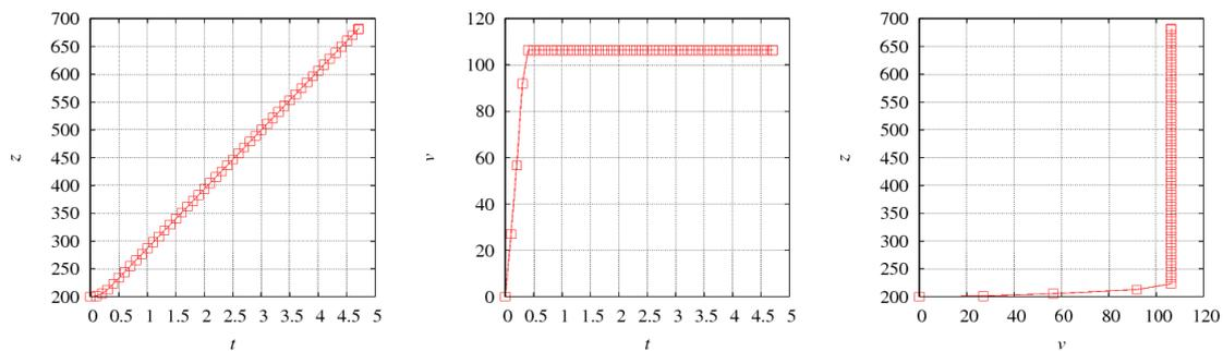
Figure D2. Fluid element position  $z$  (right) and velocity  $v$  (center) as function of time  $t$  and  $z$  against  $v$  for Well-B (discharged).
