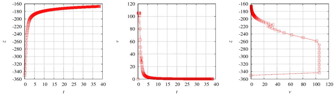
Figure D1. Fluid element position  $z$  (right) and velocity  $v$  (center) as function of time  $t$  and  $z$  against  $v$  for Well-A (not discharged).
