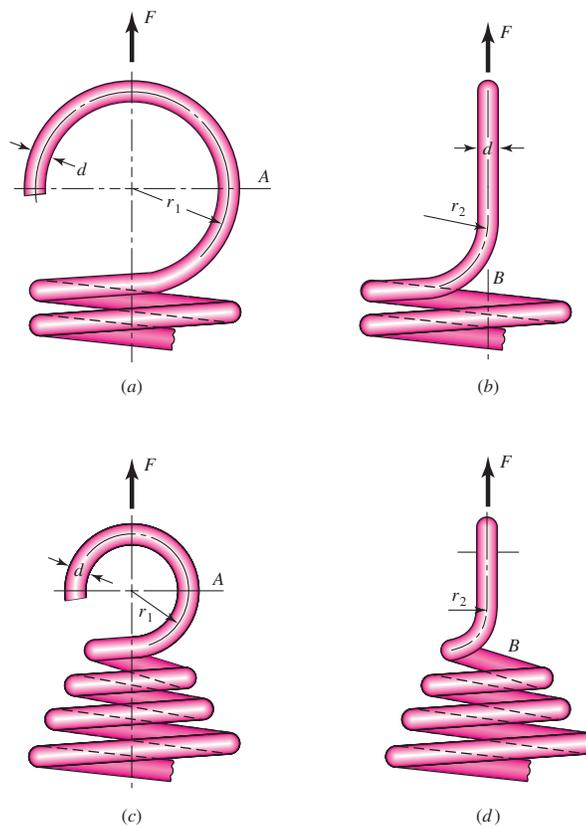
Note: Radius *r*<sub>1</sub> is in the plane of the end coil for curved beam bending stress. Radius *r*<sub>2</sub> is at a right angle to the end coil for torsional shear stress.
