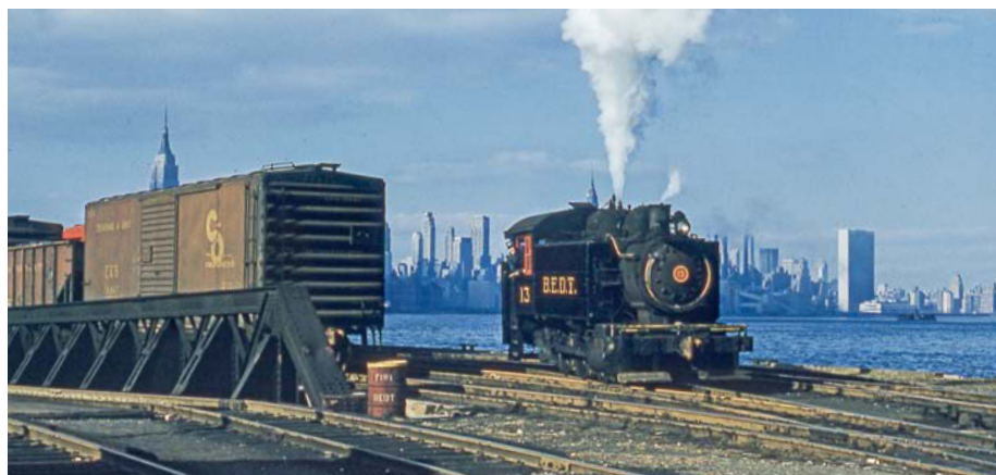
A common variation of the 0-6-0 was a tank engine 0-6-0T that carried its own fuel and water without a separate tender. This Porter-built engine is preserved at Strasburg, Pennsylvania. Richard Jay Solomon
