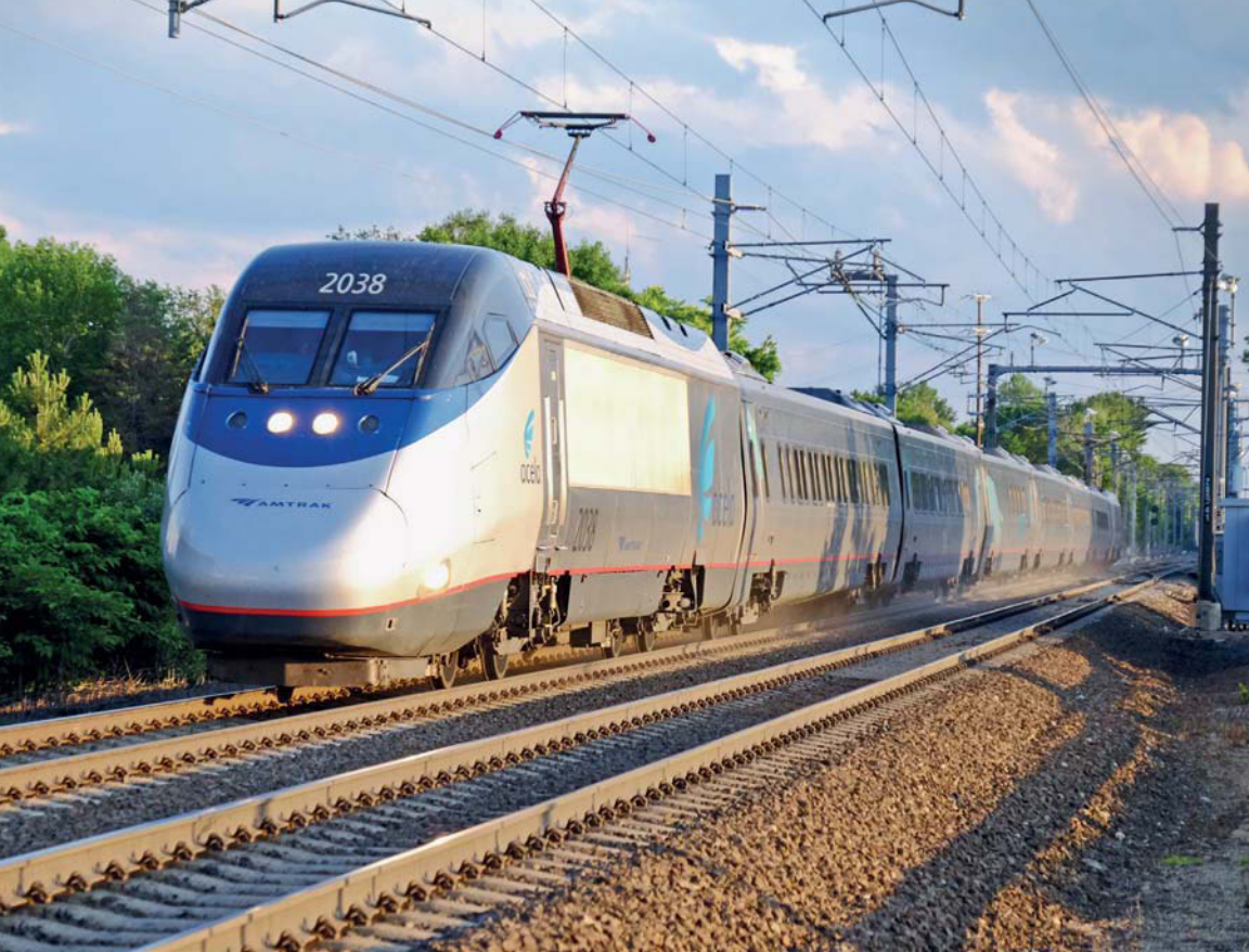
Amtrak's Acela Express High Speed Train Sets are the fastest trains in North America and are allowed to travel up to 150 mph in revenue service. Brian Solomon
