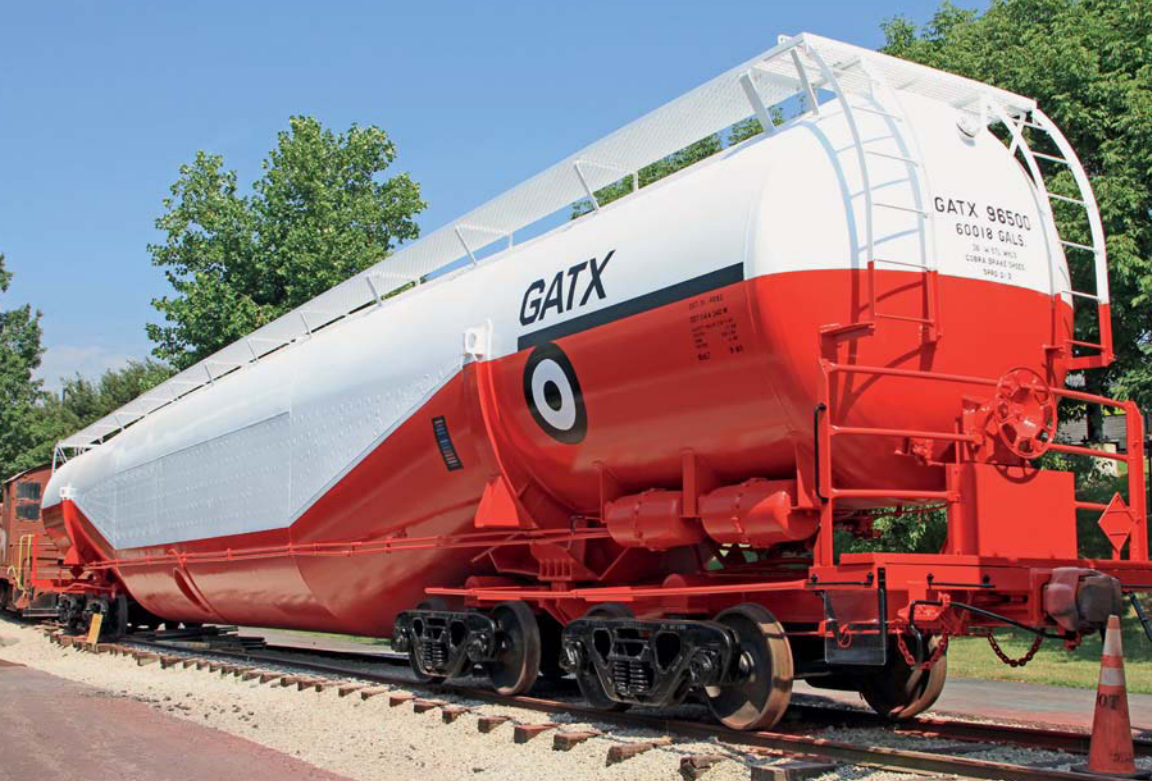
GATX is the reporting mark for General American Transportation. Exceptionally large cars such as this GATX prototype four-truck 96,500-gallon tank car are unusual in North American practice. This car is displayed at the National Museum of Transportation in St. Louis. Brian Solomon
