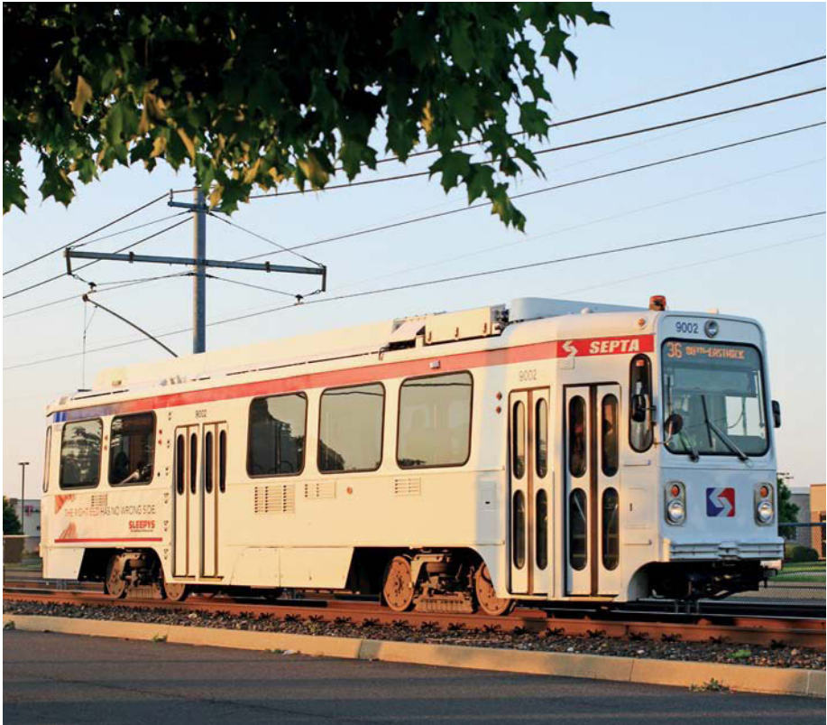
SEPTA's single-ended Kawasaki cars collect current from overhead wire using traditional trolley poles. Brian Solomon
