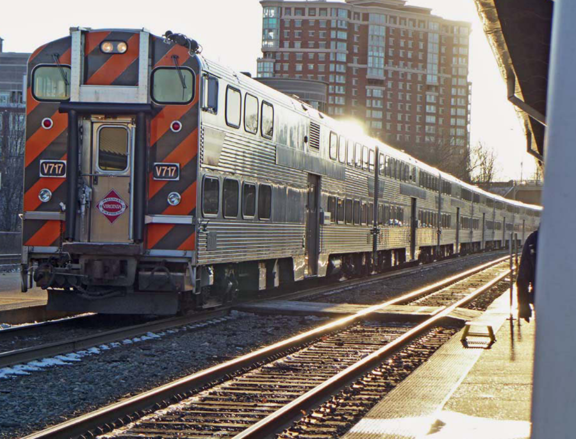
Washington, DC-based Virginia Rail Express has bought two orders of Nippon Sharyo stainless-steel gallery-style bi-level passenger cars. A VRE set working cab-car first approaches Alexandria on a January 2015 evening. Walter E. Zullig
