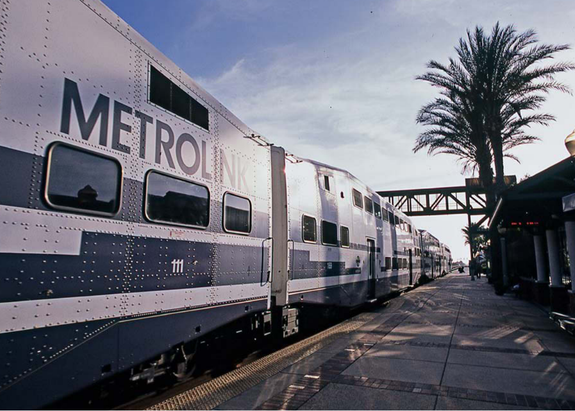
Backlighting on this set of bi-levels on Los Angeles Metrolink at Fullerton clearly shows the older style of riveted construction. Brian Solomon
