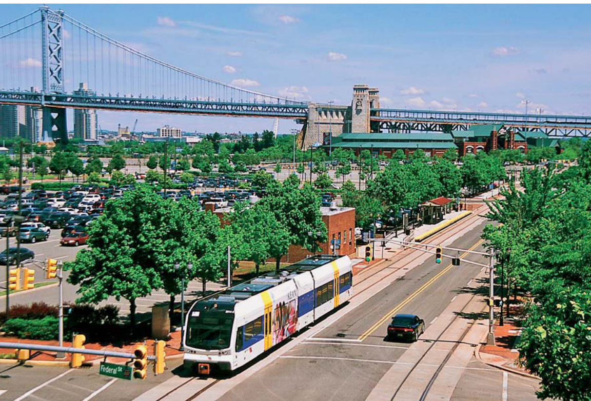
Diesel multiple units are rare in the United States, but NJ Transit's River Line service is an exception. This uses a fleet of Swiss-designed Stadler GTW 2/6. Jack May
