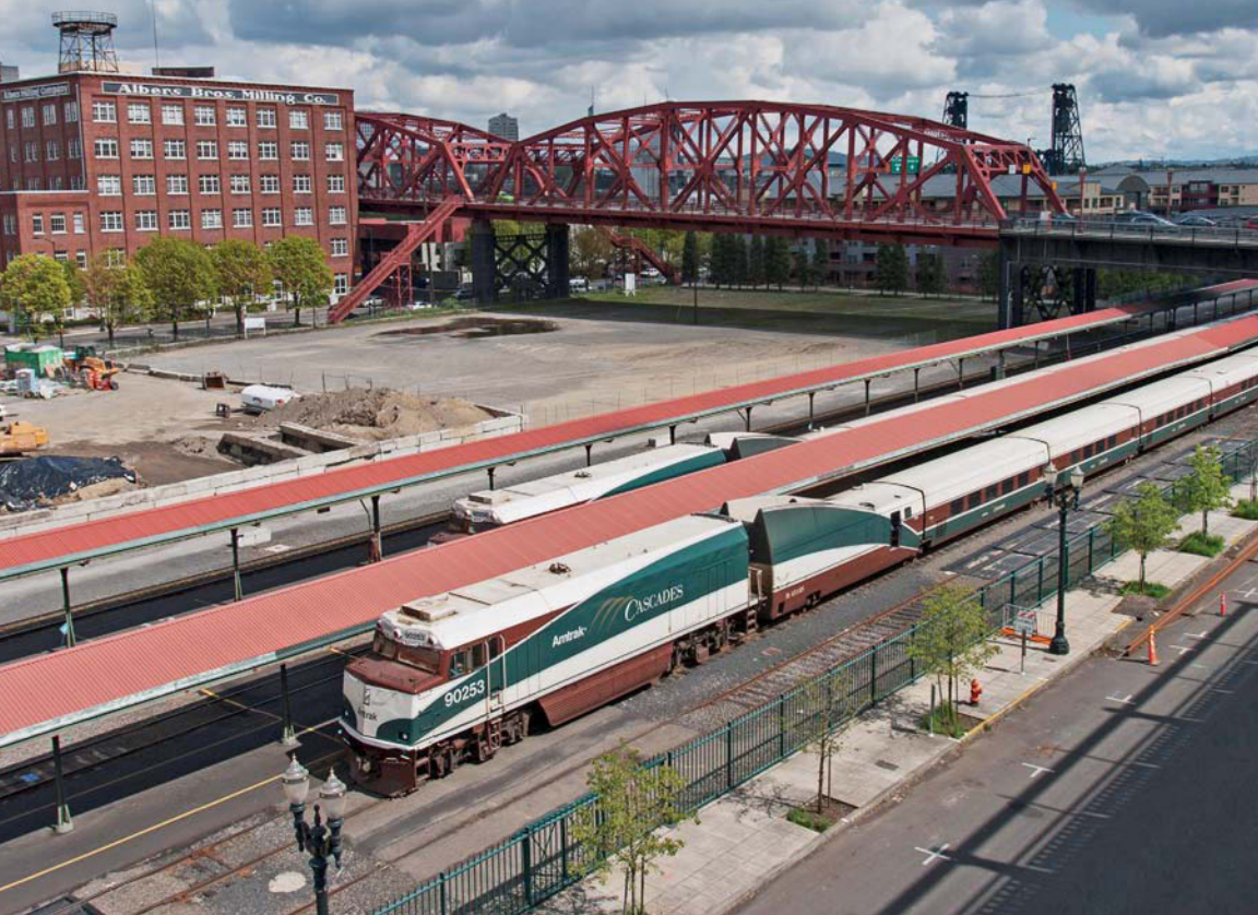
Amtrak TALGO trains wait between runs at Portland Union Station in Portland, Oregon. In the lead are Amtrak's NPCU "Cabbage" units, which had converted into unpowered cab-control cars from old F40PH diesels. Scott Lothes
