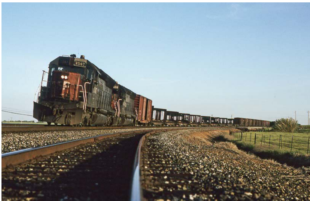
These 20-cylinder 3,600 horsepower SD45s locomotives were well suited to SP's heavy freight operations. Brian Solomon
