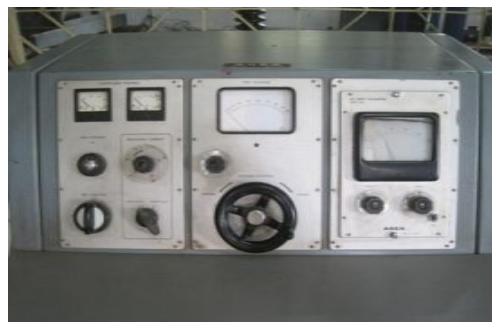
Fig.3.1. Control panel used for conducting the air breakdown test.
