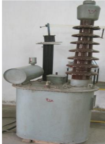
Fig.3.2. High voltage transformer used for air breakdown test.
