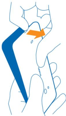
2. Make sure the contact area of the SIM is facing down, and push the SIM into the SIM slot.
