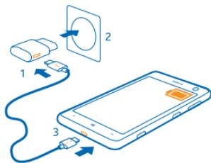
3. When the battery is full, disconnect the charger from the phone, then from the wall outlet.
