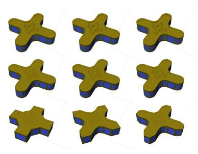
Figure 4 A matrix of 9 interval buildings' examples with identical floor area, floor-to-ceiling height, and window-to-wall ratio, but with varying number of wall sides per arc (representative sample of models used in Experiment 2, 9 sides upper right to 1 side lower left).
