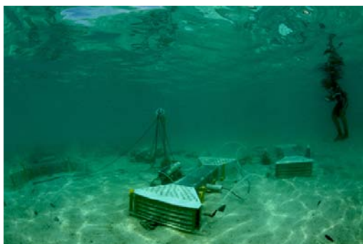
The coral proto – free ocean carbon enrichment system (CP-FOCE) deployed on Heron Island, Great Barrier Reef, Australia. Source: David Kline, Scripps.
