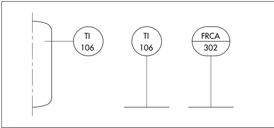
Fig. 13: Instrumentation and control tags designated according to DIN 19227 Part 1
