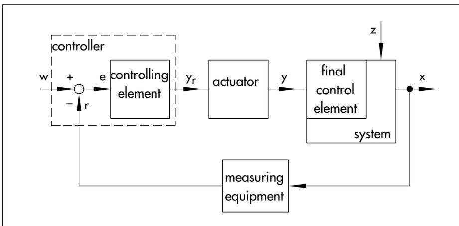
Fig. 9: Block diagram of a control loop
