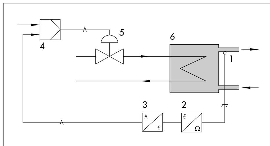
Fig. 10: Graphical symbols for describing temperature control of a heat exchanger system
