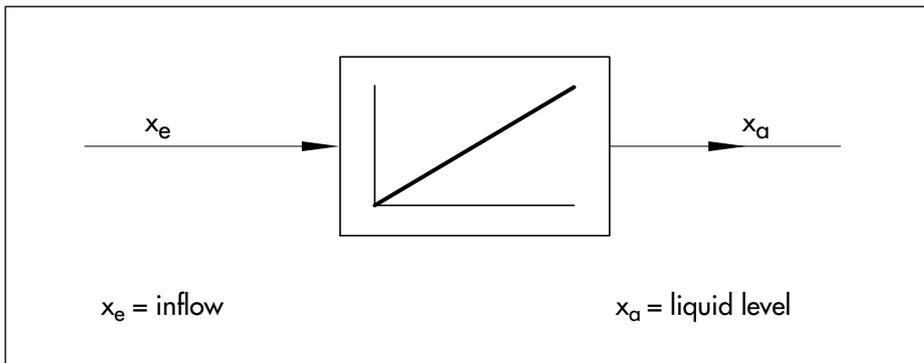
Fig. 4: Development of a liquid level over time
