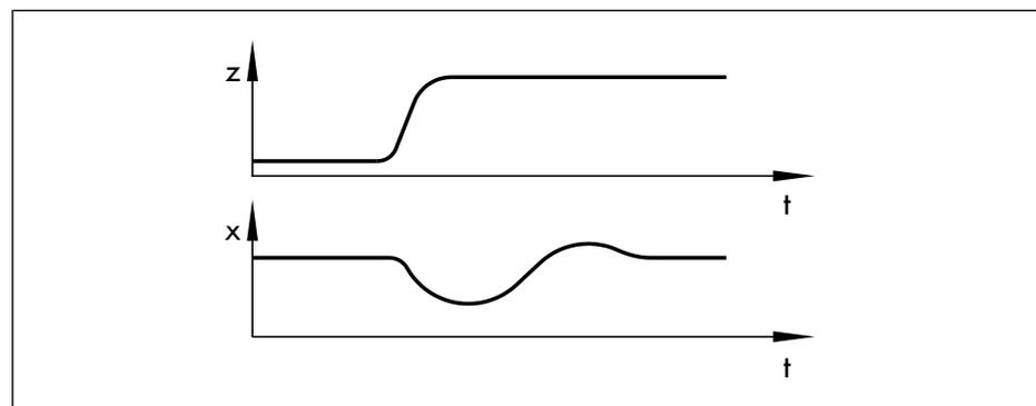
Fig. 16: Disturbance reaction
