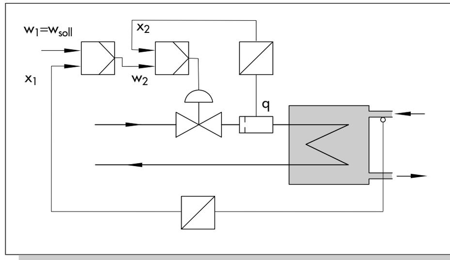
Fig. 19: Temperature control by means of cascade control
