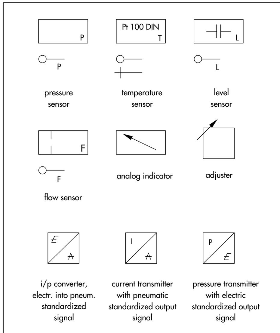
Fig. 12: Graphical symbols for sensors, transmitters, adjusters and indicators according to DIN 19227 Part 2
