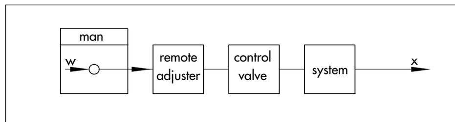
Fig. 7: Block diagram of manual open loop control
