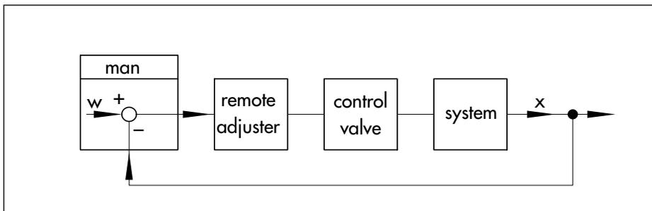
Fig. 8: Block diagram of manual closed loop control
